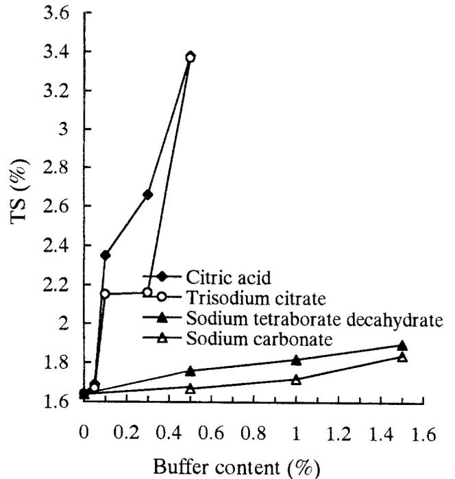
Fig. 4. Effect of buffer content on thickness swelling (TS)
