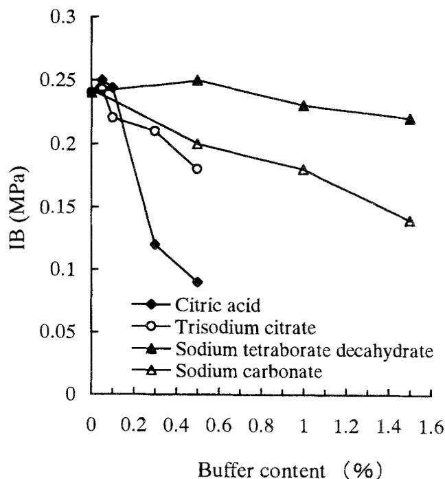
Fig. 1. Effect of buffer content on internal bond strength (IB)
