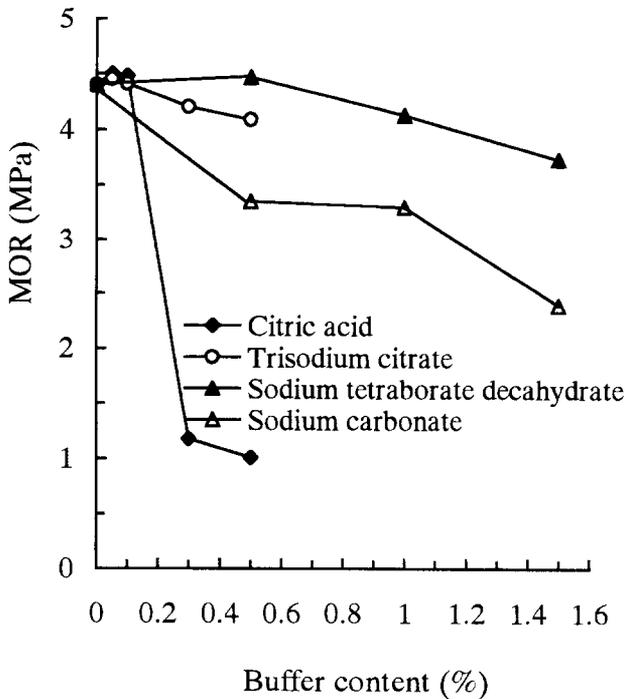
Fig. 3. Effect of buffer content on the modulus of rupture (MOR)
