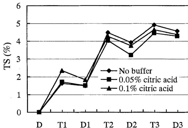
Fig. 6. Relation between the aging treatment and thickness swelling. D, air-dried condition; D1, D2, D3, oven-dried condition; T1, 24 h of soaking in water (20°C); T2, 24 h of soaking in water (70°C); T3, 4 h of boiling in water (100°C)
