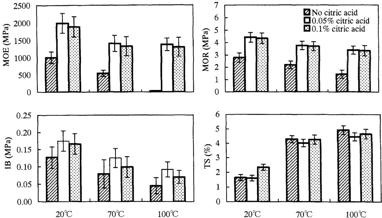
Fig. 8. Mean values and standard deviations of MOE, MOR, IB, and TS during the aging treatment
