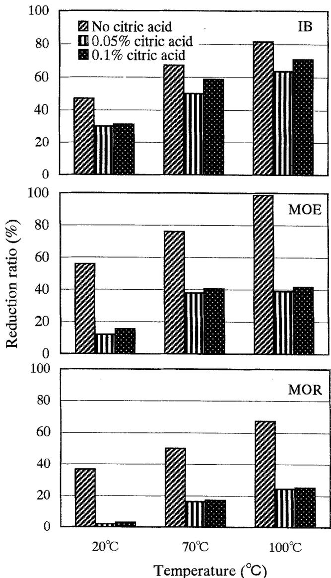
Fig. 7. Reduction ratio of IB, MOE, and MOR during the aging treatment
