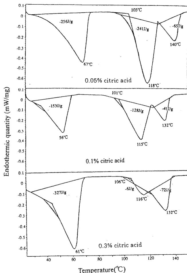
Fig. 5. Thermal analysis after addition of citric acid at concentrations of 0.05%, 0.1%, and 0.3%
