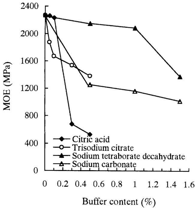
Fig. 2. Effect of buffer content on the modulus of elasticity (MOE)
