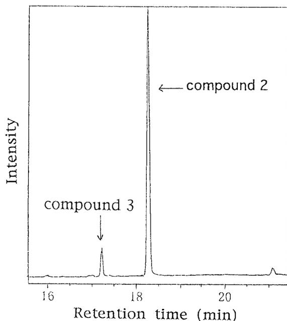
**Fig. 2.** Gas chromatographic analysis of trimethylsilane (TMS) derivative of compound 2, where a trace amount of compound 3 was obtained as an impurity
