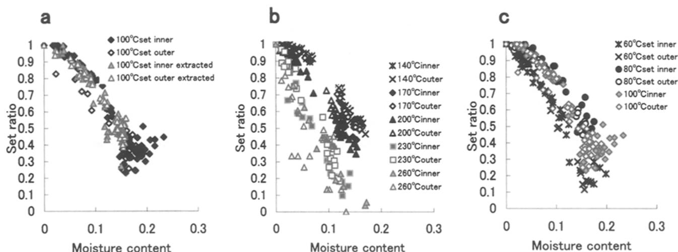
**Fig. 4.** Set ratio plotted versus moisture content. **a** Untreated and extracted specimens were set at 100°C. **b** Thermally pretreated specimens set at 100°C. **c** Specimens set at 60° and 80°C
