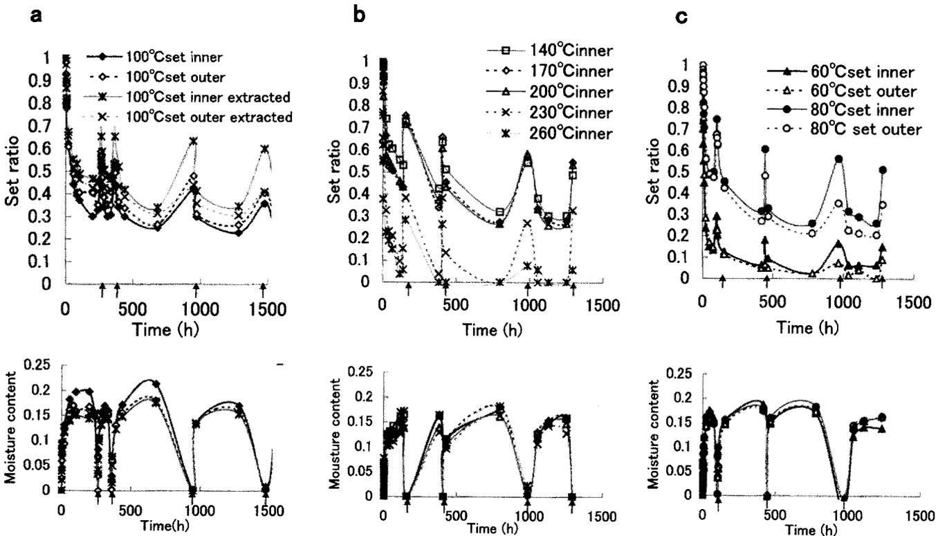
Fig. 2. Set ratios and moisture contents plotted against time when the bamboo specimens were exposed to repeated moisturizing and drying. The plotting started when the set specimens were initially exposed to humid air of 98% relative humidity (RH) at 20°C. **a** Untreated and previously extracted specimens set at 100°C. **b** Thermally pretreated specimens at 140°–260°C set at 100°C. **c** Untreated speci-
