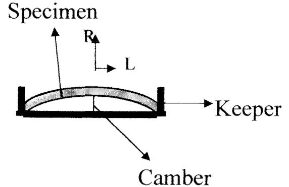
Fig. 1. Set of a bamboo specimen while bending
