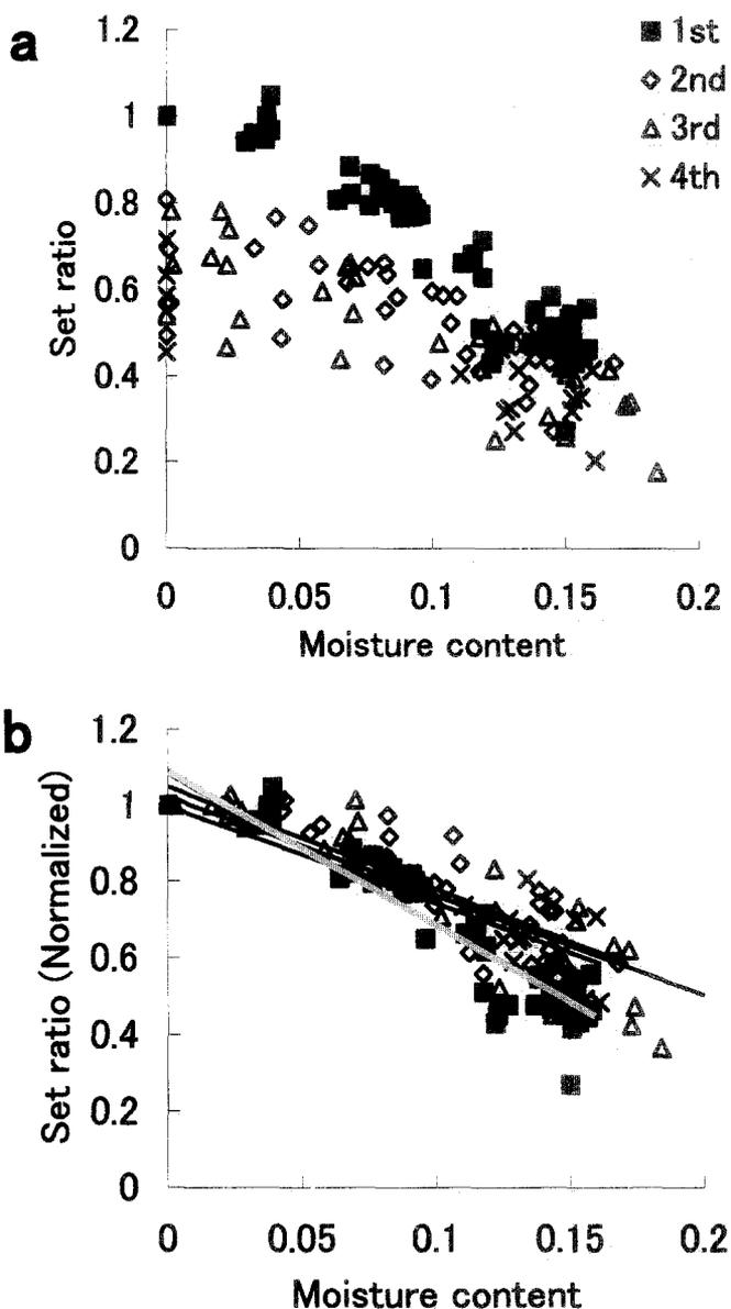
**Fig. 3.** **a** Set ratios of the first to fourth cycles were plotted versus moisture content. **b** As in **a**, but the set ratio was normalized by the initial set ratio of each cycle. *Gray line*, approximation to the first cycle; *black lines*, approximation to the second, third, and fourth cycles. As an example, only an extracted specimen from the inner layer set at 100°C is shown here
