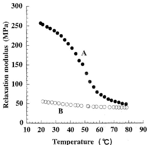
Fig. 1. Stress relaxation of wood during temperature elevation and reduction shown as the relation between relaxation modulus and temperature. A, elevation of temperature; B, reduction of temperature
