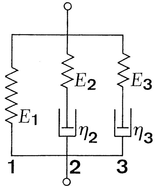
**Fig. 3.** Viscoelastic model of wood for simulation.  $E_1$ ,  $E_2$ ,  $E_3$ , moduli of elasticity;  $\eta_2$ ,  $\eta_3$ , coefficients of viscosity.  $E_2$  and  $\eta_2$  are related to moisture content of wood;  $E_3$  and  $\eta_3$  vary with temperature
