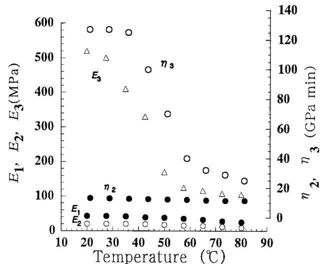
**Fig. 4.** Values of  $E_1$ ,  $E_2$ ,  $E_3$ ,  $\eta_2$ , and  $\eta_3$  for simulations. Values were the same at the same temperatures for both processes of temperature elevation and reduction
