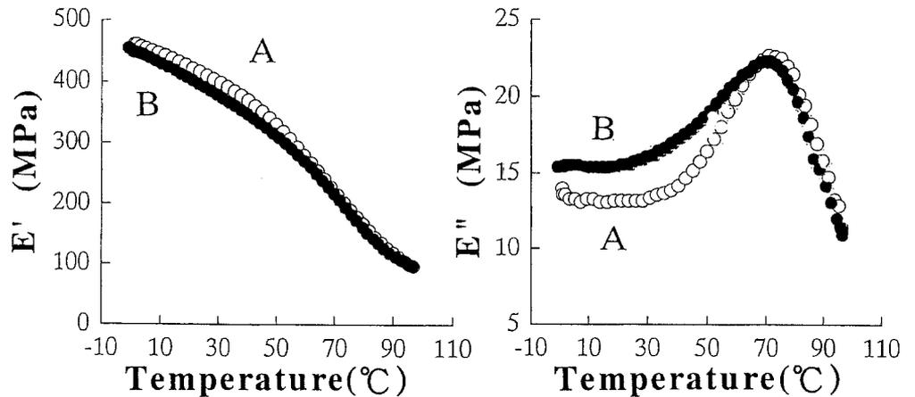
Fig. 10. Changes in  $E''$  for green wood (left) and water-saturated wood after drying once (right) during elevation and reduction of temperature. A, elevation of temperature; B, reduction of temperature
