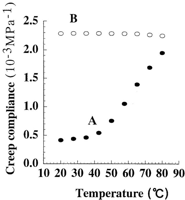
**Fig. 2.** Changes in creep compliance during the elevation and reduction of temperature. A, elevation of temperature; B, reduction of temperature
