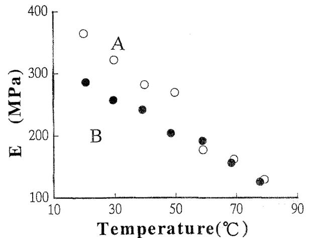
Fig. 6. Temperature dependence of Young's modulus  $E$  during bending. A, elevation of temperature; B, reduction of temperature
