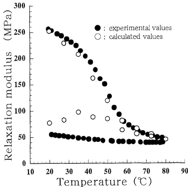
Fig. 5. Comparison of experimental and simulated values when the elements were given the values shown in Fig. 4
