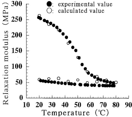
Fig. 8. Comparison of experimental and simulated values when the elements were assigned the values shown in Fig. 7
