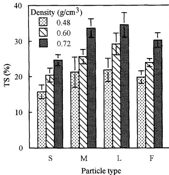
Fig. 6. Effect of particle shape on thickness swelling (TS) of the particleboard after vacuum-pressure soak and oven-dried exposure
