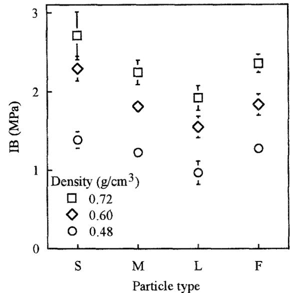
Fig. 7. Effect of particle shape on the internal bond (IB) strength of the particleboard
