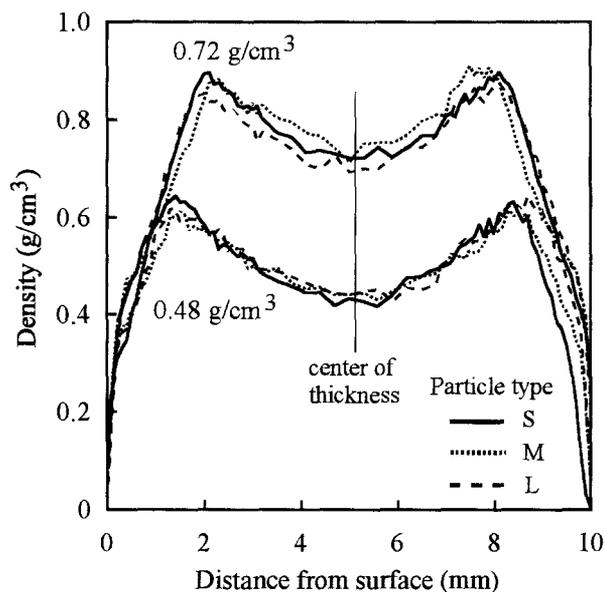
Fig. 4. Density profile of the particleboards
