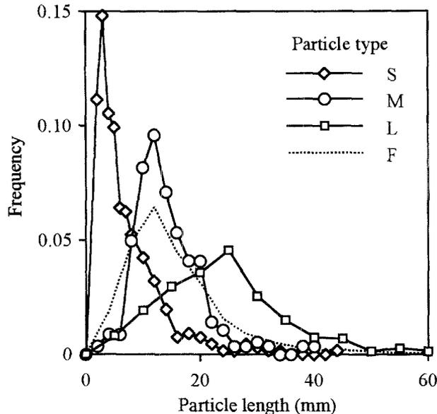
**Fig. 2.** Distribution of particle length as determined by the image analysis. F, mixture of S, M, and L mesh
