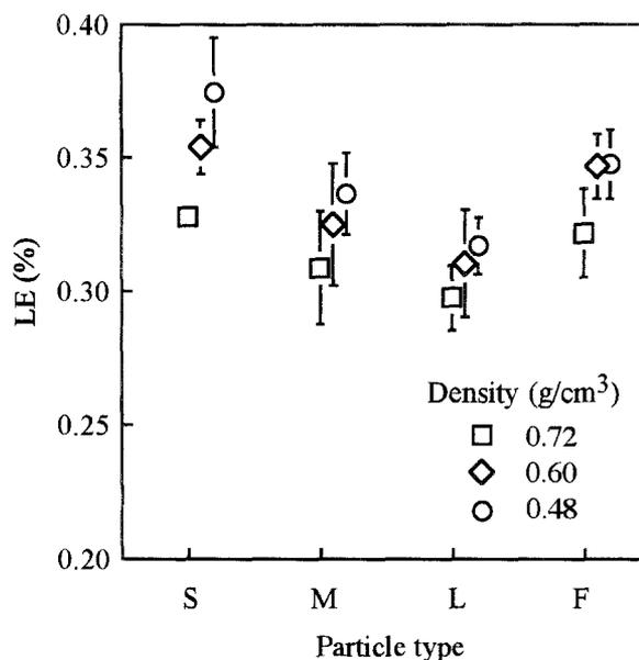
Fig. 5. Effect of particle shape on linear expansion (LE) of particleboard at 40°C and 90% relative humidity
