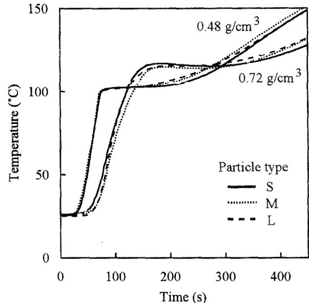
**Fig. 3.** Temperature behavior at the center of the mat with time after press closure
