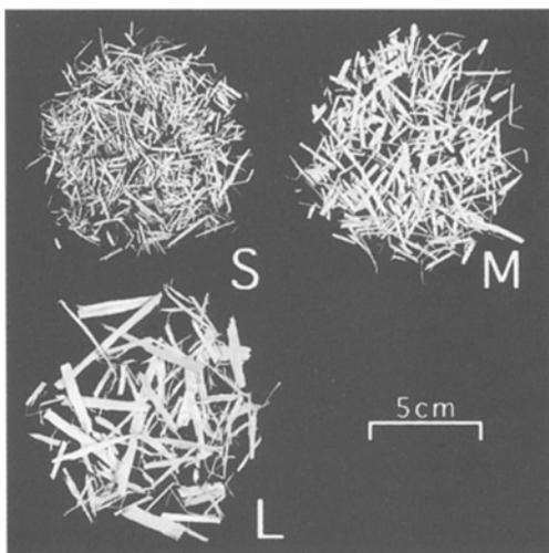
**Fig. 1.** Three types of particles prepared by hammer-milling hinoki strands. S, +6.5 mesh; M, -6.5 + 10.0 mesh; L, -10 mesh
