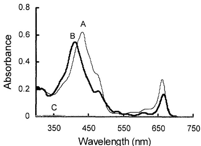
**Fig. 4.** Ultraviolet-visible spectra of chlorophyll extracted with acetone from the treated bamboo by ultrasonics. A, pretreated; B,  $\text{H}_3\text{PO}_4$ -treated; C,  $\text{H}_3\text{PO}_4\text{-CrO}_3$ -treated
