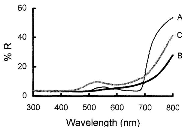
**Fig. 1.** Diffuse reflectance ultraviolet-visible (UV-VIS) spectra of ma bamboo after CrO<sub>3</sub>-H<sub>3</sub>PO<sub>4</sub> two-step treatment. A, pretreated; B, CrO<sub>3</sub>-treated; C, CrO<sub>3</sub>-H<sub>3</sub>PO<sub>4</sub>-treated
