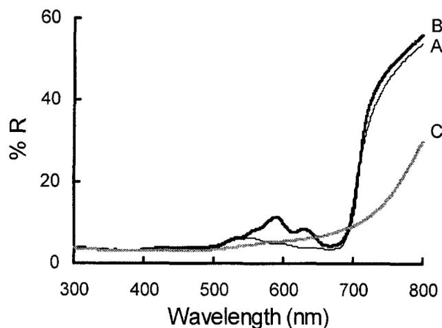
**Fig. 2.** Diffuse reflectance UV-VIS spectra of ma bamboo after  $\text{H}_3\text{PO}_4\text{-CrO}_3$  two-step treatment. A, pretreated; B,  $\text{H}_3\text{PO}_4$ -treated; C,  $\text{H}_3\text{PO}_4\text{-CrO}_3$ -treated
