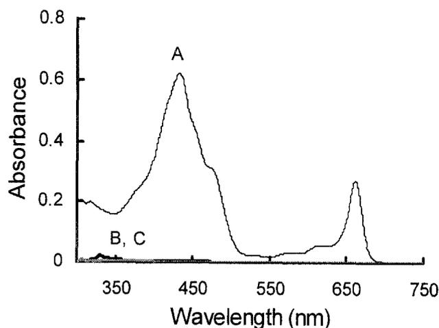
**Fig. 3.** Ultraviolet-visible spectra of chlorophyll extracted with acetone from the treated bamboo by ultrasonics. A, pretreated; B,  $\text{CrO}_3$ -treated; C,  $\text{CrO}_3\text{-H}_3\text{PO}_4$ -treated
