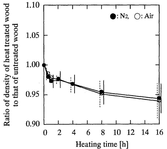
**Fig. 7.** Changes in density caused by heat treatment. The same specimens were used before and after treatment. *Filled circles*, specimens heat treated in N<sub>2</sub> gas; *open circles*, specimens heat treated in air. *Solid lines at the right side of the filled circles and dashed lines at the left side of the open circles* are the standard deviation
