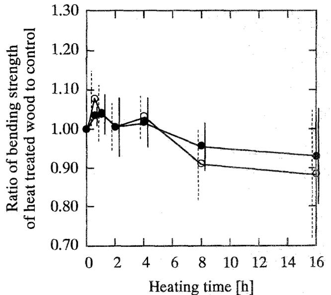
Fig. 11. Changes in bending strength due to heat treatment. Values are the average of  $\sigma/\sigma_c$  in each group.  $\sigma$ , bending strength of heat-treated wood;  $\sigma_c$ , bending strength of control. Refer to Fig. 7 for explanation of symbols
