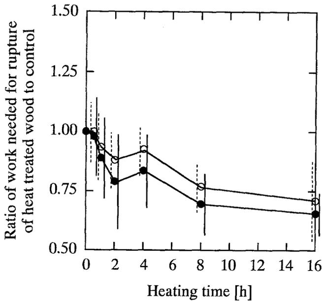
**Fig. 12.** Changes in work needed for rupture due to heat treatment. Values are the average of  $W_{04}/W_{04c}$  in each group.  $W_{04}$ , work needed for rupture of heat-treated wood;  $W_{04c}$ , work needed for rupture of control. Refer to Fig. 7 for explanation of symbols
