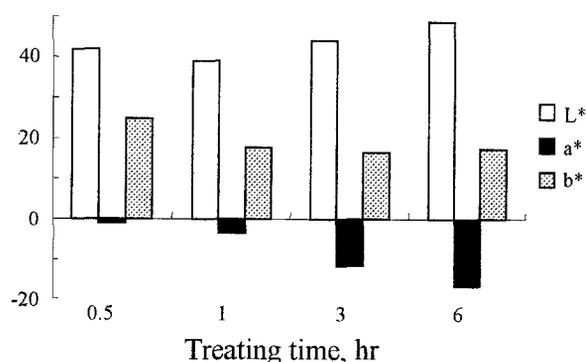
Fig. 3. Color changes of ma bamboo as a function of CP treating time
