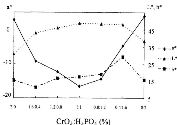
Fig. 2. Influence of CrO<sub>3</sub>/H<sub>3</sub>PO<sub>4</sub> ratios in CP on the color of ma bamboo
