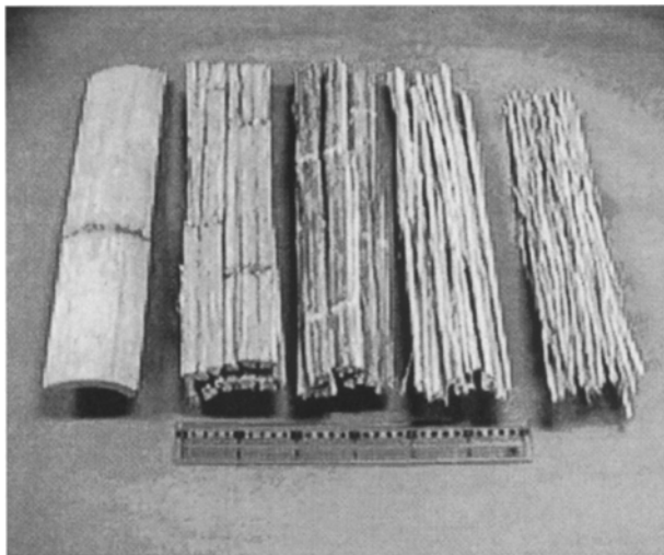
Fig. 1. Bamboo zephyr strand from moso bamboo. From left to right: bamboo culm and bamboo zephyr strands with diameters of 9.5, 4.7, 2.8, and 1.5 mm, respectively
