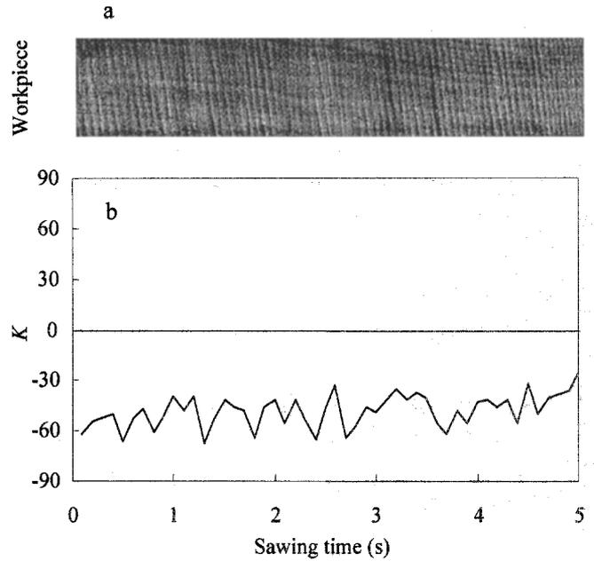
Fig. 9. Situation of sawn surface of the workpiece (a) and the behavior of  $K$  corresponding to the sawn surface (b). Washboard appeared on whole sawn surface
