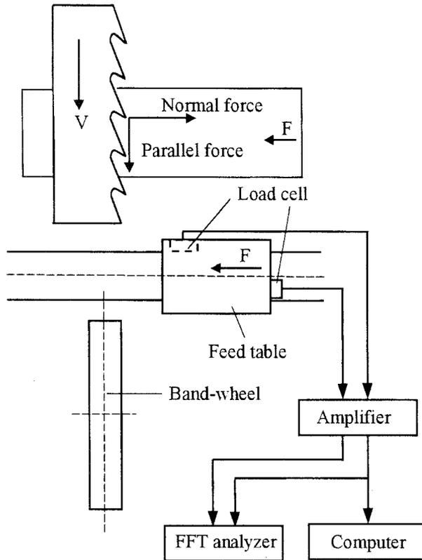
Fig. 1. Experiment setup.  $V$ , sawing direction;  $F$ , feed direction; FFT, fast Fourier transform
