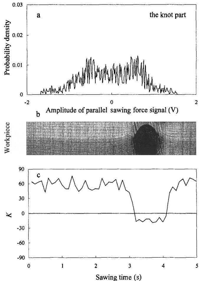
**Fig. 11.** **a** Curve of probability density distribution of the parallel sawing force to the knot part. **b** Situation of the sawn surface of the workpiece including the knot. **c** Behavior of  $K$  corresponding to the sawn surface. Washboarding appeared only on the knot part of the sawn surface
