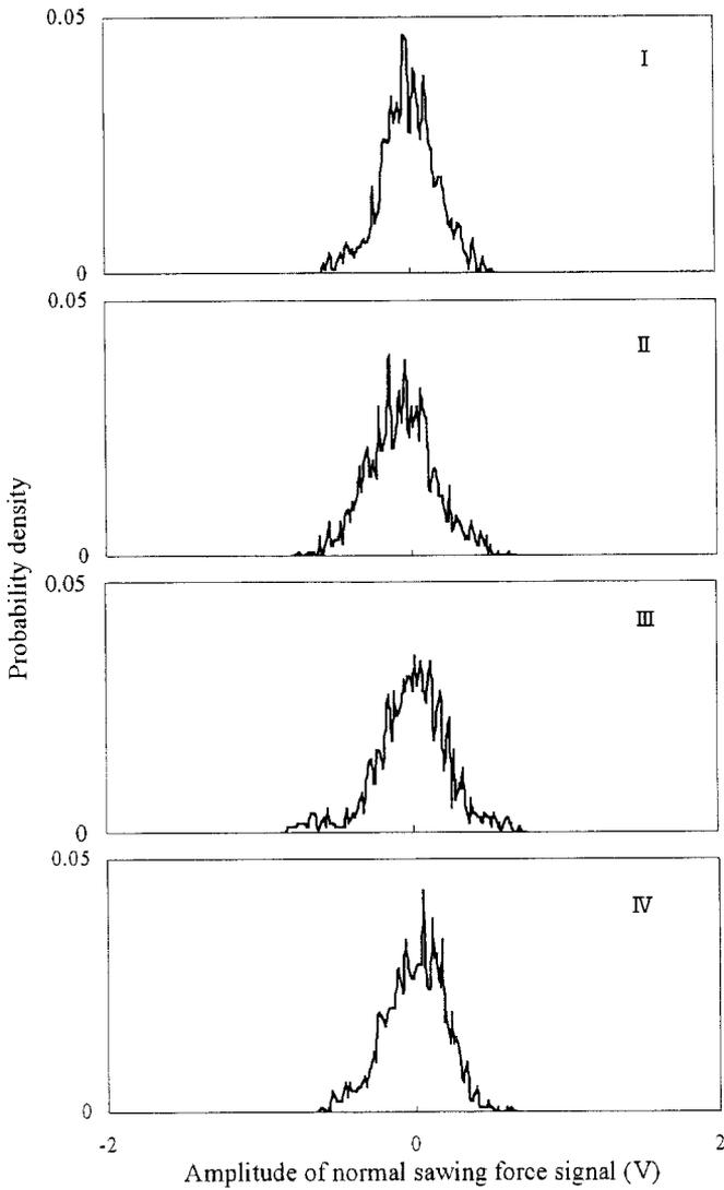
Fig. 7. Curves of probability density function of the normal sawing force for four parts of the sawn surface. I to IV, shown in Fig. 2
