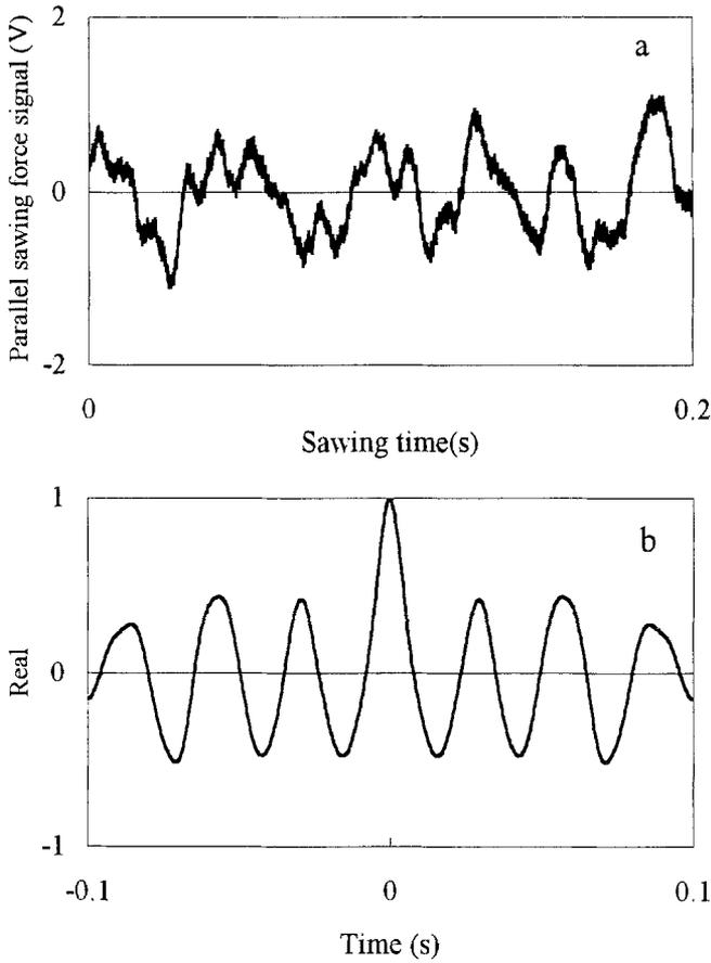
**Fig. 4.** Parallel sawing force signal (a) and its autocorrelation function (b) for part III in Fig. 2
