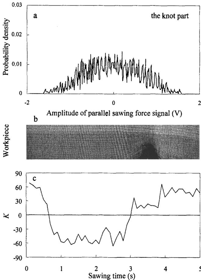
**Fig. 10.** **a** Curve of probability density distribution of the parallel sawing force to the knot part. **b** Situation of the sawn surface of the workpiece including the knot. **c** Behavior of  $K$  corresponding to the sawn surface. Washboarding did not appear on the knot part of the sawn surface
