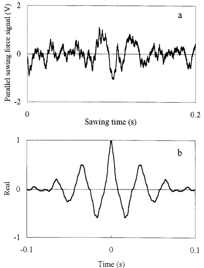
Fig. 3. Parallel sawing force signal (a) and its autocorrelation function (b) for part I in Fig. 2
