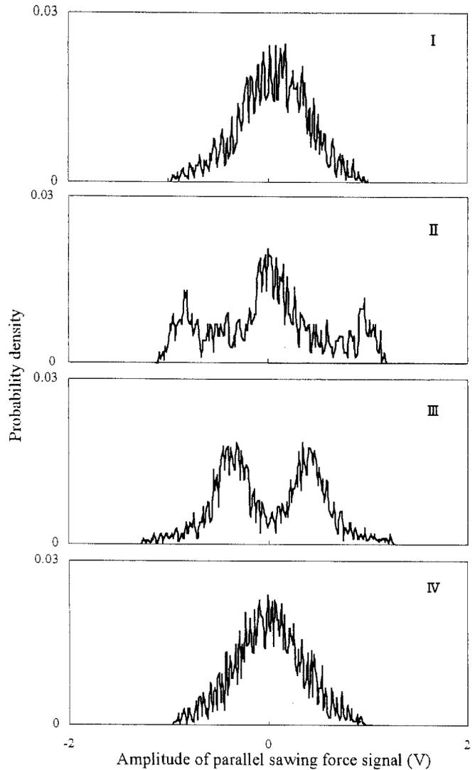
Fig. 6. Curves of probability density function of the parallel sawing force for four parts of the sawn surface, I to IV, shown in Fig. 2
