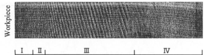
Fig. 2. Sawn surface of a workpiece divided into four parts. Parts I and IV show normal sawn surfaces. Part II has the appearance of a washboard. Part III has a washboard pattern
