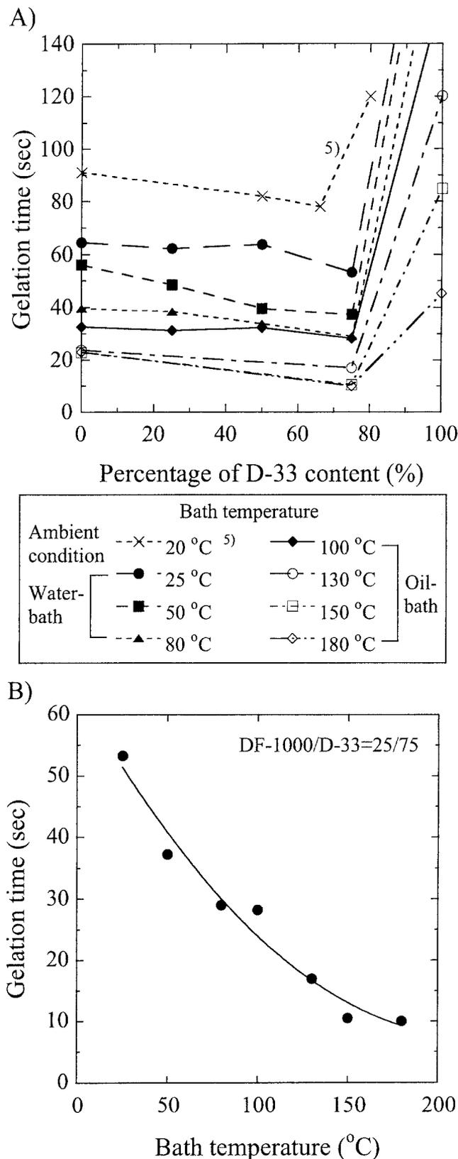
**Fig. 8.** **A** Effects of resin mix ratio and bath temperature on gelation time. The number "5" is a reference number. **B** Relations between gelation time and bath temperature at DF-1000/D-33 25:75
