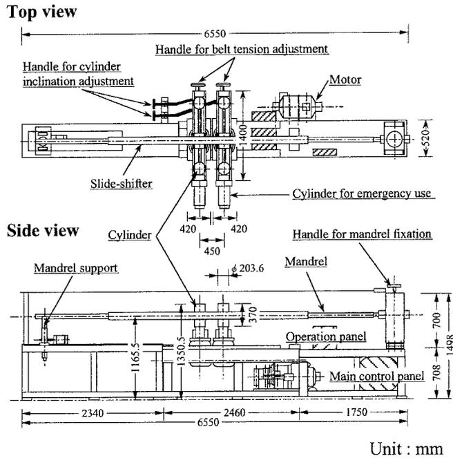
Fig. 1. Parts of the spiral-winder
