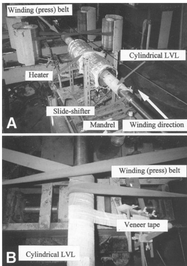
**Fig. 3.** Manufacturing process of cylindrical laminated veneer lumber (LVL). **A** Appearance of spiral-winder and pilot installed cylindrical heater. **B** Close-up view
