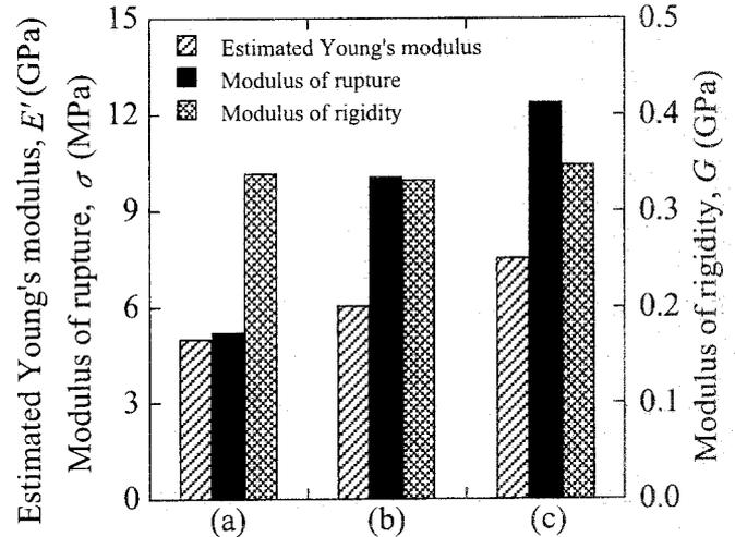
Fig. 13. Comparison of bending performance of cylindrical LVL (four-ply) manufactured by various combinations of veneer width and press time. Refer to Fig. 12 for an explanation of (a), (b), and (c)
