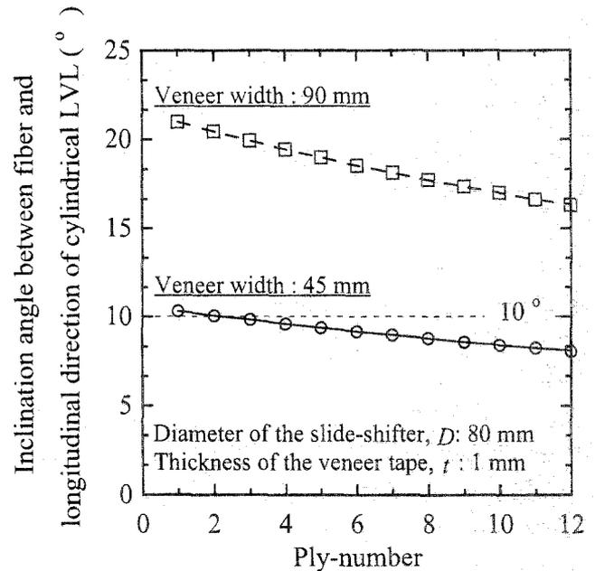
**Fig. 6.** Relations between ply number and calculated fiber inclination angle to the longitudinal direction of cylindrical LVL
