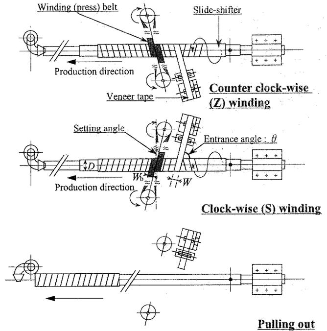
Fig. 2. Relations among production direction, the entrance direction of the veneer tape, and the setting angle of the cylinder
