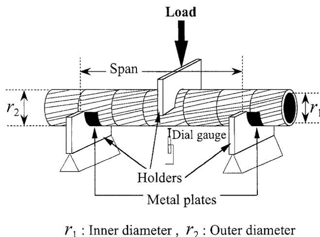
Fig. 7. Setup for the static bending test of cylindrical LVL
