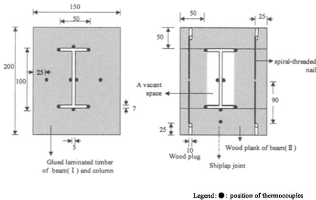
Fig. 1. Location of thermocouples (units are millimeters)
