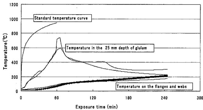
Fig. 2. Temperature of flanges, webs, and the 25 mm depth in the beam (I)
