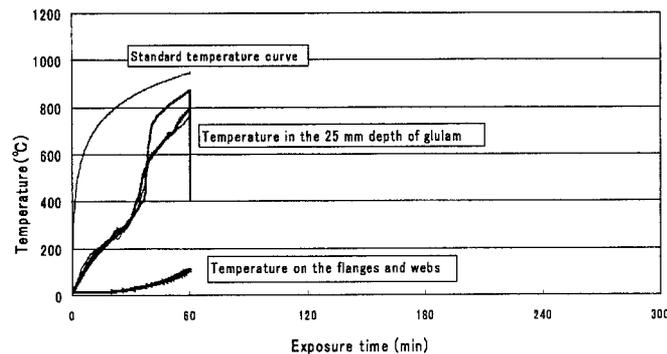
Fig. 3. Temperature of flanges, webs, and the 25 mm depth in the column
