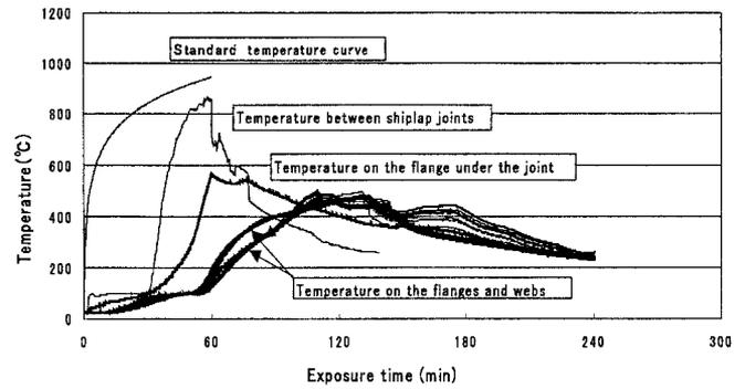
Fig. 4. Temperature of flanges, webs, and the 25 mm depth in the beam (II)
