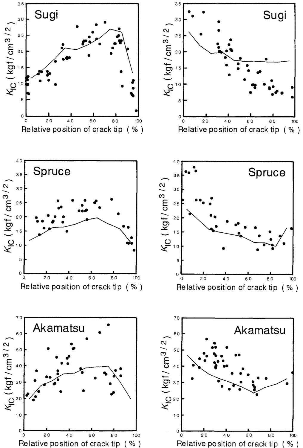
The results of measurements of acoustic emission (AE) and fractography of spruce in our previous report<sup>2</sup> were compared with the results from the present work and can be summarized as follows. When the degree of stress concentration was small, an AE of a small amplitude was gradually generated, and intrawall failure was clearly observed at the fracture surface that was considered to be formed before the crack initiation. On the other hand, when
