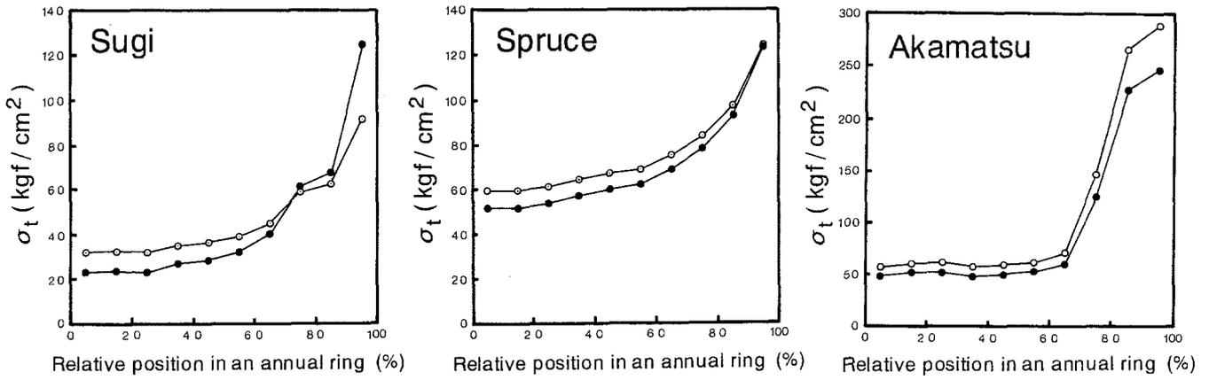
Fig. 7. Distributions of the predicted tensile strength in a single annual ring. Filled circles,  $\sigma_{Tt}$ ; open circles,  $\sigma_{Rt}$
