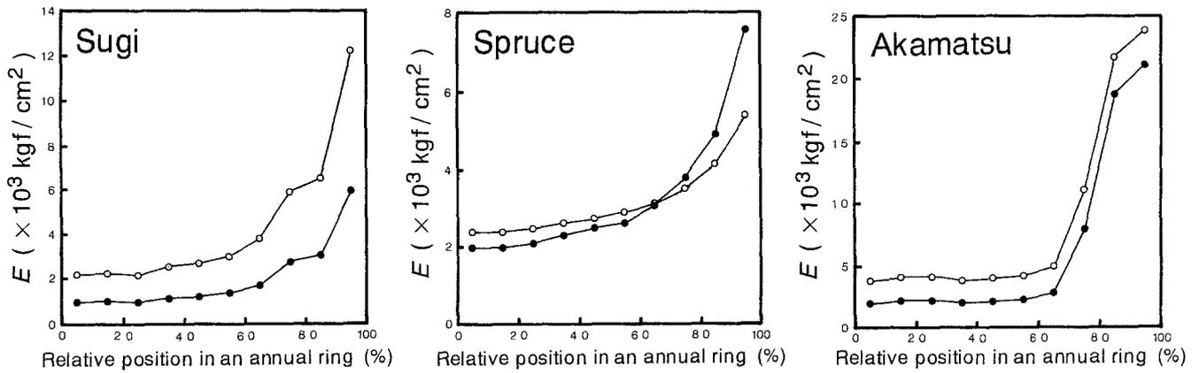
Fig. 5. Distributions of the predicted modulus of elasticity in a single annual ring. Filled circles,  $E_T$ ; open circles,  $E_R$
