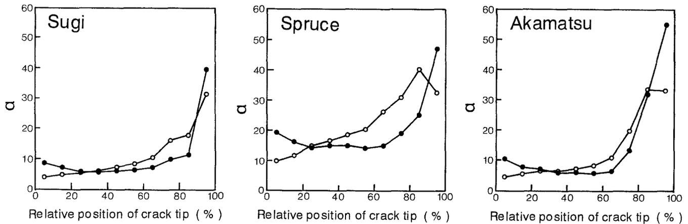
Fig. 10. Relations between the stress concentration factor ( $\alpha$ ) and the location of a crack tip in a single annual ring. Filled circles, pith-side notched; open circles, bark-side notched
