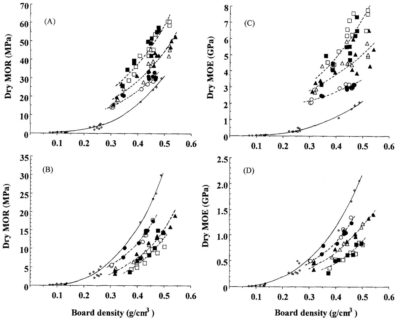
**Fig. 1.** Dry bending properties of sandwich panels and low-density fiberboards. Dry MOR in parallel (A) and perpendicular (B) directions and dry MOE in parallel (C) and perpendicular (D) directions. Veneer thickness of sandwich panels are 0.55 mm (circles), 1.0 mm (triangles),
