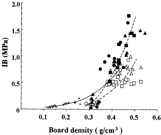
**Fig. 3.** Internal bond strength of sandwich panels and low-density fiberboards. Veneer thickness of sandwich panels are 0.55 mm (circles), 1.0 mm (triangles), and 2.0 mm (squares). Core layer resin contents of sandwich panels are 10% (open symbols) and 30% (filled symbols). Small open diamonds, low-density fiberboard
