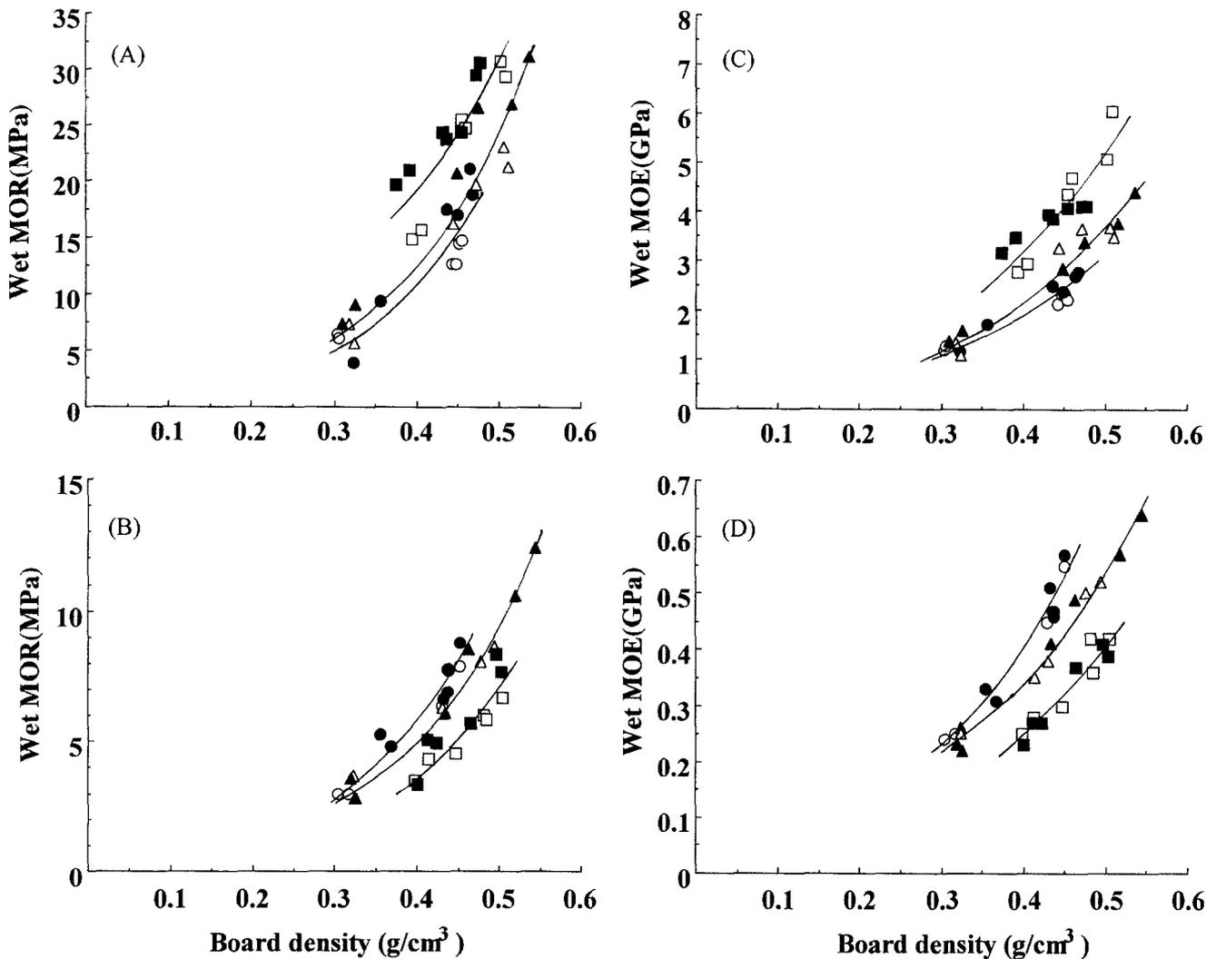
**Fig. 2.** Wet bending properties of sandwich panels. Wet MOR in parallel (A) and perpendicular (B) directions and wet MOE in parallel (C) and perpendicular (D) directions. Veneer thicknesses of sandwich pan-
