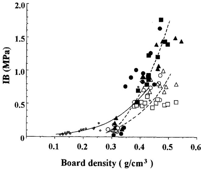
**Fig. 3.** Internal bond strength of sandwich panels and low-density fiberboards. Veneer thickness of sandwich panels are 0.55 mm (circles), 1.0 mm (triangles), and 2.0 mm (squares). Core layer resin contents of sandwich panels are 10% (open symbols) and 30% (filled symbols). Small open diamonds, low-density fiberboard
