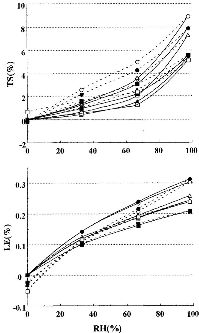
**Fig. 6.** Linear expansion (LE) and thickness swelling (TS) of sandwich panels with a mean density of  $0.4\text{ g/cm}^3$  in relation to the relative humidity (RH) during moisture absorption (solid lines) and desorption (dotted lines) processes. Veneer thickness of sandwich panels are 0.55 mm (circles), 1.0 mm (triangles), and 2.0 mm (squares). Core layer resin contents of sandwich panels were 10% (open symbols) and 30% (filled symbols)
