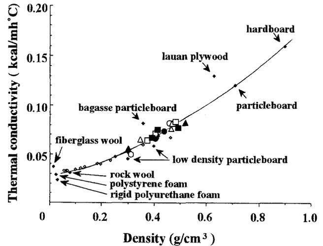
**Fig. 7.** Thermal conductivity of sandwich panels and other materials. Veneer thicknesses of sandwich panels were 0.55 mm (circles), 1.0 mm (triangles), and 2.0 mm (squares). Core layer resin contents of sandwich panels were 10% (open symbols) and 30% (filled symbols). Small open diamonds, low-density fiberboard
