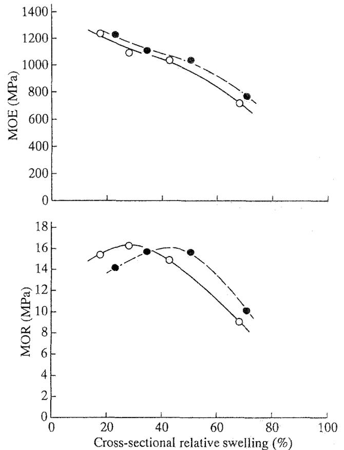
**Fig. 7.** Difference in *MOE* and *MOR* for wood moisture-conditioned for 4 weeks by the adsorption process (*open symbols*) and by the desorption process from a moisture content below the FSP (*solid symbols*) as a function of cross-sectional relative swelling
