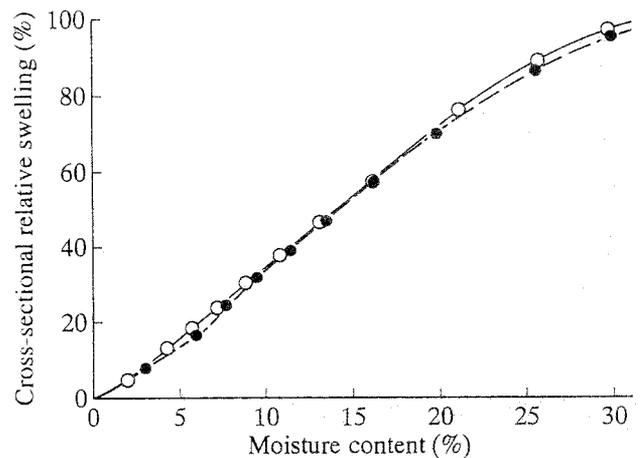
Fig. 4. Difference in cross-sectional relative swelling between wood moisture-conditioned for 50 weeks during the adsorption process (open symbols) and that during the desorption process from a water-saturated state (solid symbols)
