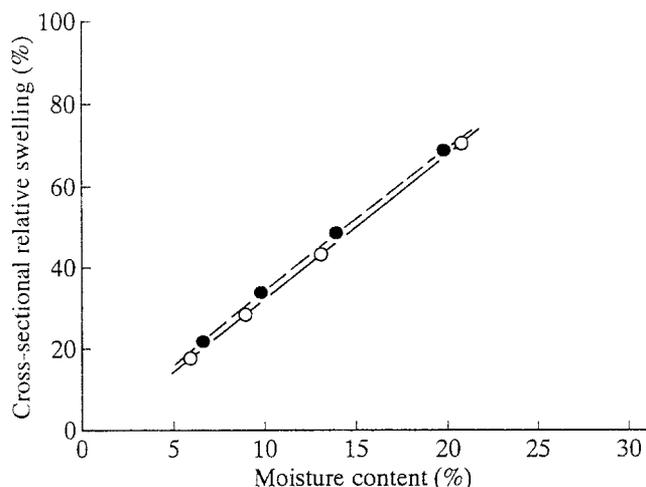
**Fig. 5.** Difference in cross-sectional relative swelling between wood moisture-conditioned for 9 weeks during the adsorption process (*open symbols*) and that during the desorption process from a moisture content slightly below the fiber saturation point (FSP) (*solid symbols*)
