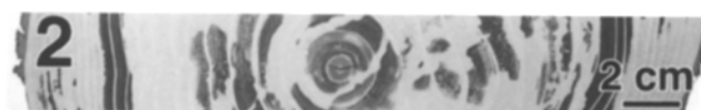
Fig. 2. Soft X-ray photograph of a sample section showing irregularly distributed wet areas in the heartwood. Tree no. 11-540, clone name Kujii 38, MC is 204%
