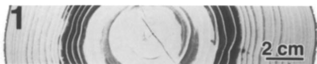
Fig. 1. Soft X-ray photograph of a sample section showing regularly distributed wet areas in the heartwood. Tree no. 11-761, clone name Chichibu (Ken) 6, MC (mean moisture content of the heartwood) is 213%. [NOTE: All soft X-ray photographs in this paper are represented in negative. Thus, darker portions in the photographs show portions of low X-ray absorption and little water presence in the sample section; lighter portions show high X-ray absorption and much water]
