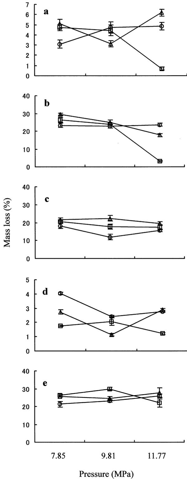
**Fig. 1.** Effect of the interaction between treatment temperature and pressure on the mass loss of medium-density fiberboard (a), hardwood plywood (b), softwood plywood (c), particleboard (d), and oriented strand board (e) with *Trametes versicolor*. Open circles, triangles, and squares represent treatment temperatures of 35°C, 45°C, and 55°C, respectively. Vertical lines represent standard errors
