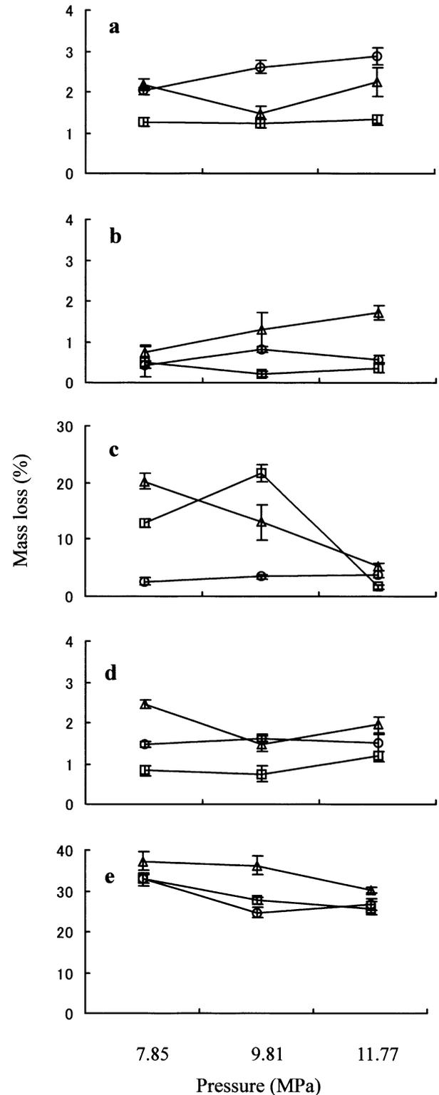
**Fig. 2.** Effect of the interaction between treatment temperature and pressure on the mass loss of medium-density fiberboard (a), hardwood plywood (b), softwood plywood (c), particleboard (d), and oriented strand board (e) with *Fomitopsis palustris*. Open circles, triangles, and squares represent treatment temperatures of 35°C, 45°C, and 55°C, respectively. Vertical lines represent standard errors
