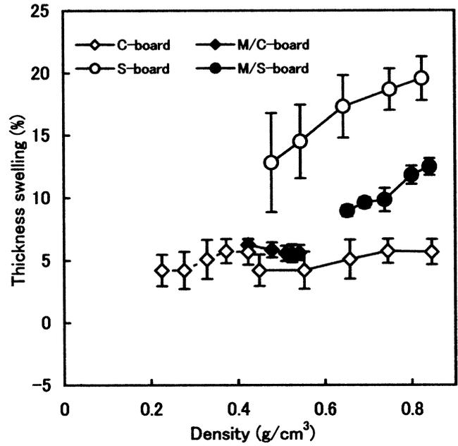
**Fig. 9.** Relation between thickness swelling and density of 20-mm-type C-board, M/C-board, S-board, and M/S-board. The densities of C-board (*dotted line*) and M/C-board were their apparent densities
