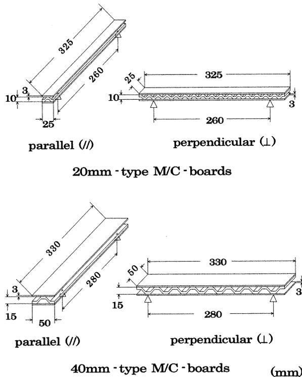
**Fig. 1.** Dimensions of parallel and perpendicular specimens of medium-density fiberboard (MDF)-reinforced corrugated particleboard (M/C-boards) and the span lengths of bending tests
