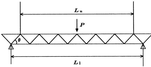
Fig. 5. Truss model for structural analysis of perpendicular specimens of composite board.  $L_u$  and  $L_l$ , lengths of the upper and lower chords, respectively;  $P$ , load;  $\theta$ , angle of the diagonal member
