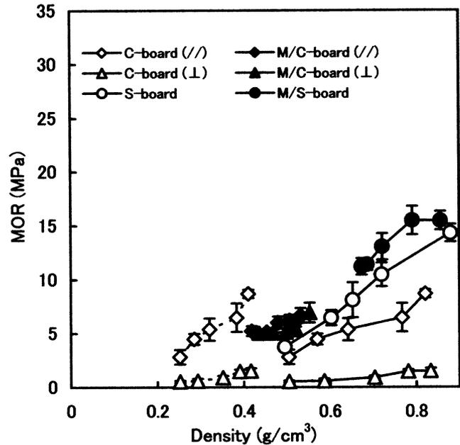
Fig. 7. Relation between MOR in the wet condition and the density of 20-mm-type C-board, M/C-board, S-board, and M/S-board. The densities of C-boards (dotted lines) and M/C-boards were their apparent densities
