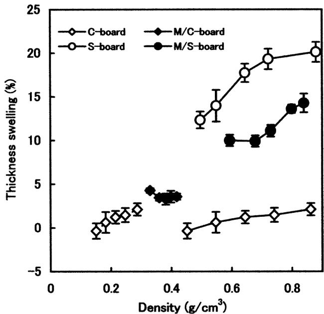
**Fig. 10.** Relation between the thickness swelling and density of 40-mm-type C-board, M/C-board, S-board, and M/S-board. The densities of C-board (*dotted line*) and M/C-board were the apparent densities
