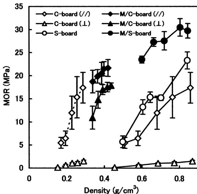
**Fig. 4.** Relation between *MOR* and density of 40-mm-type C-board, M/C-board, S-board, and M/S-board. The densities of C-boards (*dotted lines*) and M/C-boards were their apparent densities.
