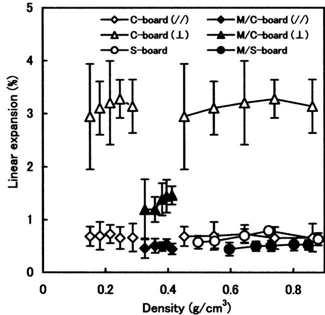
**Fig. 12.** Relation between linear expansion and the densities of 40-mm-type C-board, M/C-board, S-board, and M/S-board. The densities of C-boards (*dotted line*) and M/C-boards were their apparent densities
