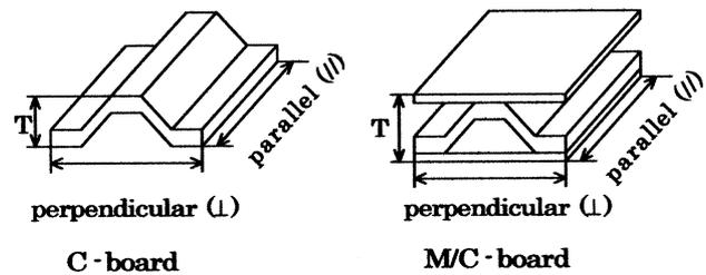
**Fig. 2.** Measuring directions for thickness swelling ( $T$ ) and linear expansion (parallel, perpendicular) of corrugated particleboard (C-board) and M/C board
