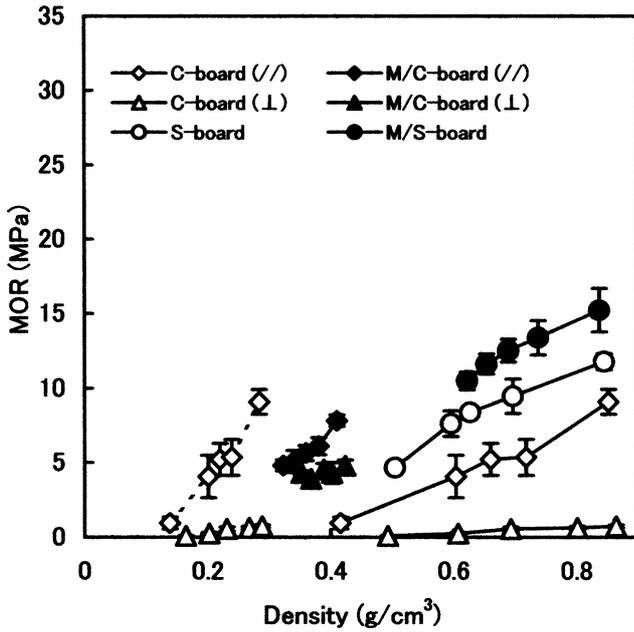
**Fig. 8.** Relation between MOR in the wet condition and the density of 40-mm-type C-board, M/C-board, S-board, and M/S-board. The densities of C-boards (*dotted lines*) and M/C-boards were their apparent densities
