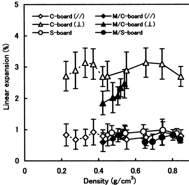
**Fig. 11.** Relation between linear expansion and density of 20-mm-type C-board, M/C-board, S-board, and M/S-board. The densities of C-boards (*dotted lines*) and M/C-boards were their apparent densities
