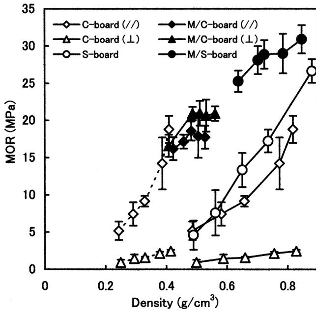
**Fig. 3.** Relation between modulus of rupture (*MOR*) and density of 20-mm-type C-board, M/C-board, standard flat-type particle board (*S-board*), and M/S-board. The densities of C-boards (*dotted lines*) and M/C-boards were their apparent densities.
