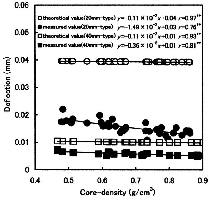
Fig. 6. Relations between the deflection and core-density of perpendicular specimens of M/C-board as the truss beam
