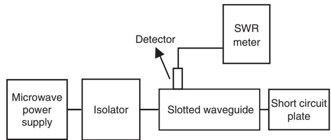
Fig. 1. Equipment used for the determination of the dielectric properties of the material
