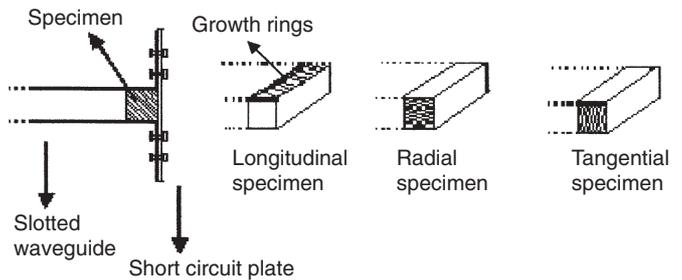
Fig. 2. Placement of the test specimens in the waveguide
