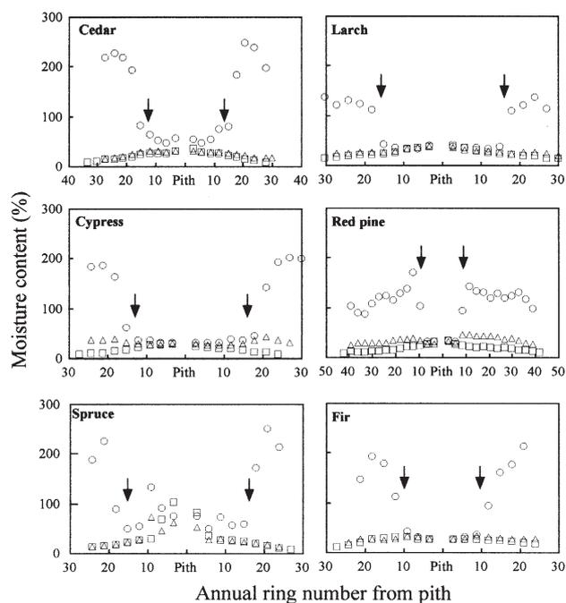
**Fig. 1.** Changes in moisture content as a result of smoke heating of six Japanese softwoods. Open circles, control; open triangles, 100-h treatment; open squares, 200-h treatment. Arrows indicate boundary between heartwood and sapwood
