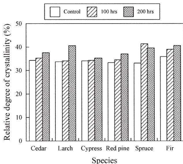
**Fig. 2.** Changes in relative degree of crystallinity as a result of smoke-heating of six Japanese softwoods
