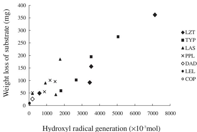
**Fig. 6.** Correlation between hydroxyl radical generation in wood cultures and the rate of degradation of wood in glucose cultures
