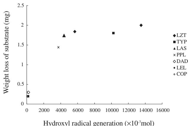
**Fig. 8.** Correlation between hydroxyl radical generation in wood or glucose cultures and the rate of degradation of a lignin model compound in wood or glucose cultures
