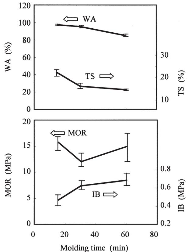
**Fig. 5.** Effect of molding time on MOR, IB, WA, and TS of the boards. The molding temperature was 180°C and the board density was 0.7 g/cm<sup>3</sup>
