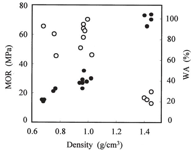
Fig. 3. Modulus of rupture (MOR, filled circles) and water absorption (WA, open circles) of the boards as a function of their density. The molding temperature and time were  $180^\circ\text{C}$  and 15 min, respectively
