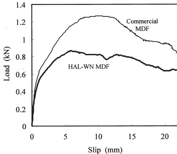
**Fig. 6.** Averaged load-slip curves of the nailed joints in single-shear tests for commercial medium-density fiberboard (MDF) and hardwood acetic acid-waste newspaper (HAL-WN) MDF
