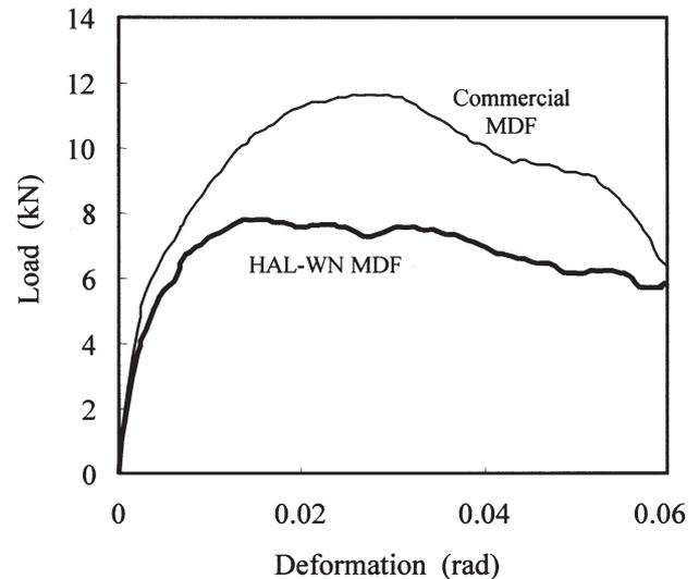
**Fig. 7.** Simulated load-deformation curves of nailed shear walls of commercial MDF and HAL-WN MDF
