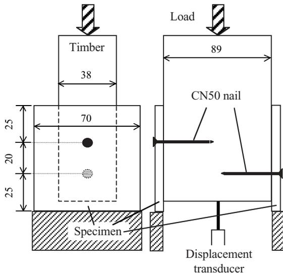
Fig. 1. An experimental single-shear test of nailed joint
