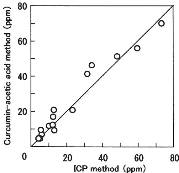
**Fig. 3.** Relationship between boron content determined by the ICP method and by the curcumin-acetic acid method
