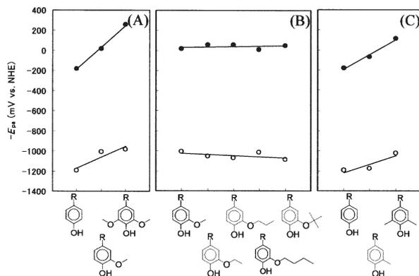
**Fig. 3.** Effect of substituents on the anodic peak potentials ( $E_{pa}$ ) of monolignols (A), monoalkoxy series (group A) (B), methyl series (group B) (C). Lines are to guide reader's eye. High  $-E_{pa}$  value means high oxidizability. Filled circles, phenolate form; open circles, phenol form; R-,  $-\text{CH}=\text{CHCH}_2\text{OH}$
