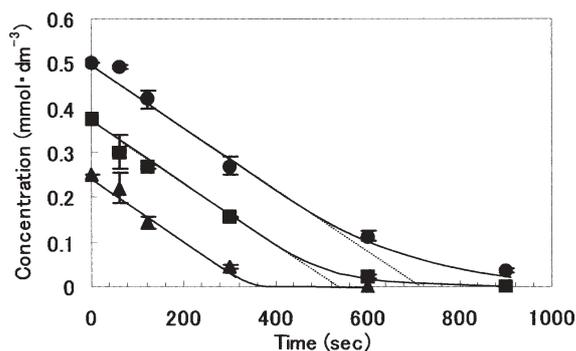
**Fig. 4.** Reaction curves for oxidation of coniferyl alcohol at different initial concentrations using HRP–H<sub>2</sub>O<sub>2</sub> as the oxidant. *Circles*, initial concentration 0.5 mmol dm<sup>-3</sup>, *n* = 2; *squares*, initial concentration 0.375 mmol dm<sup>-3</sup>, *n* = 4; *triangles*, initial concentration 0.25 mmol dm<sup>-3</sup>, *n* = 3. Error bars show standard error
