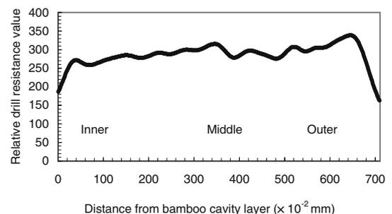
**Fig. 3.** Drilling resistance record measured from a bamboo sample
