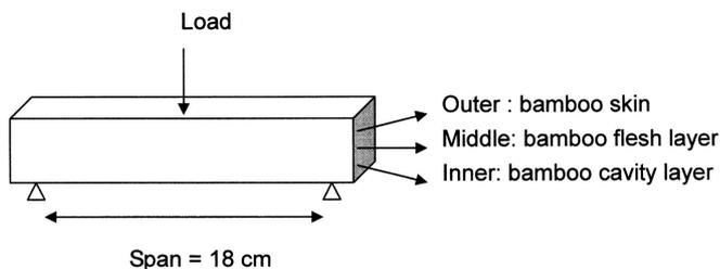
**Fig. 2.** Configuration of the static bending test for bamboo lamina
