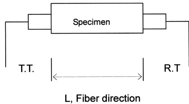
**Fig. 1.** Measurement method for ultrasonic velocity and dynamic modulus of elasticity of bamboo lamina.  $L$ , Length of specimen;  $T.T.$ , transmitting transducer;  $R.T.$ , receiving transducer
