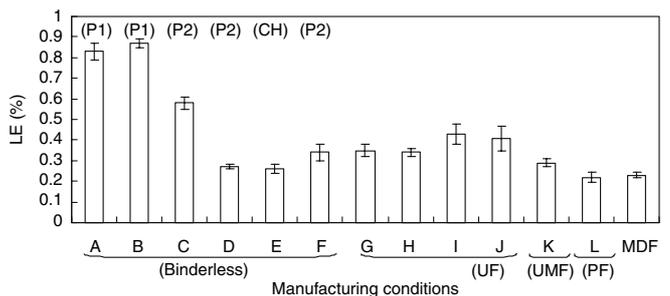
**Fig. 6.** Linear expansion (*LE*) of boards manufactured under various conditions. For details of manufacturing conditions *A-F* and *G-L*, see Tables 3 and 4, respectively
