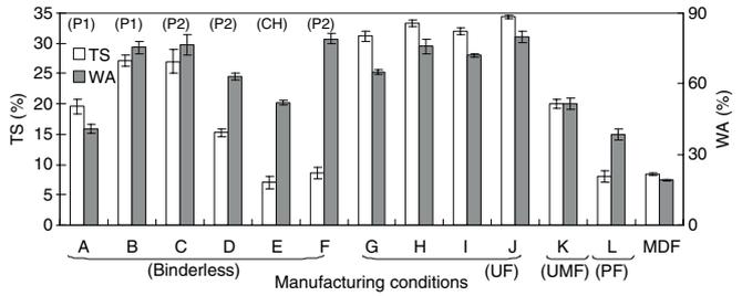
**Fig. 5.** TS and WA of boards manufactured under various conditions. For details of manufacturing conditions *A-F* and *G-L*, see Tables 3 and 4, respectively
