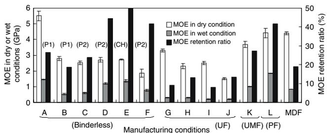
**Fig. 3.** MOE in dry and wet conditions and the retention ratio of boards manufactured under various conditions. For details of manufacturing conditions *A-F* and *G-L*, see Tables 3 and 4, respectively
