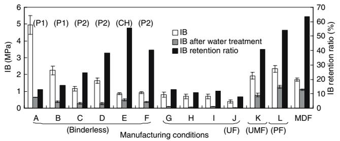
**Fig. 4.** IB, IB after water treatment, and the retention ratio of the boards manufactured under various conditions. For IB after water treatment, the IB values were determined after soaking in water (20°C) for 24h and then drying. For details of manufacturing conditions *A-F* and *G-L*, see Tables 3 and 4, respectively
