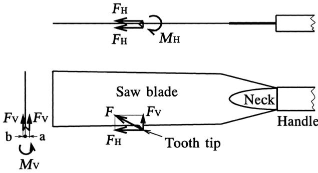
Fig. 1. The moments placed on the teeth by the cutting resistances when the left saw set is larger than the right
