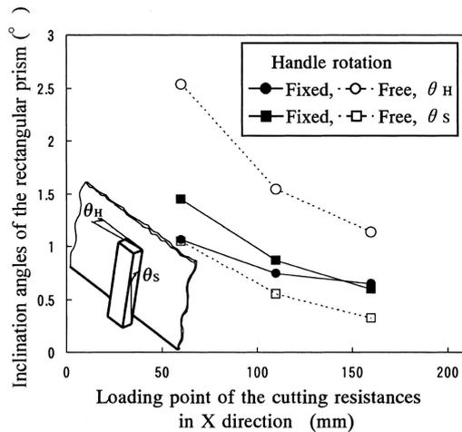
Fig. 11. Inclination of the rectangular prism by FEM calculation
