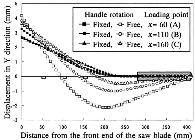
Fig. 9. Displacement of the top end of the saw by FEM calculation
