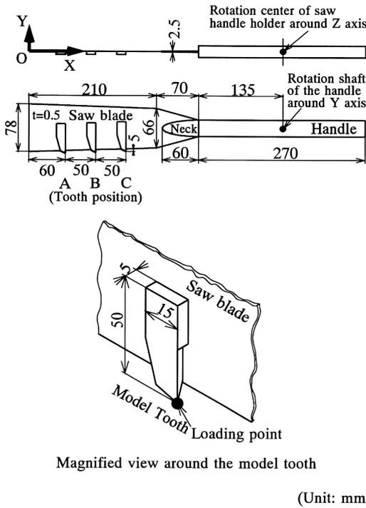
Fig. 2. Saw blade with model tooth
