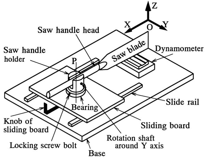
Fig. 3. Experimental device
