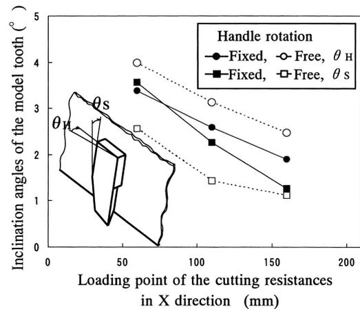
Fig. 7. Experimental inclination of the the model tooth.  $\theta_H$ , inclination angle of model tooth from X direction in top view;  $\theta_S$ , inclination angle of model tooth from a normal line in operator view
