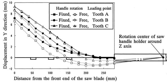
Fig. 5. Experimental displacement of the top end of the saw blade
