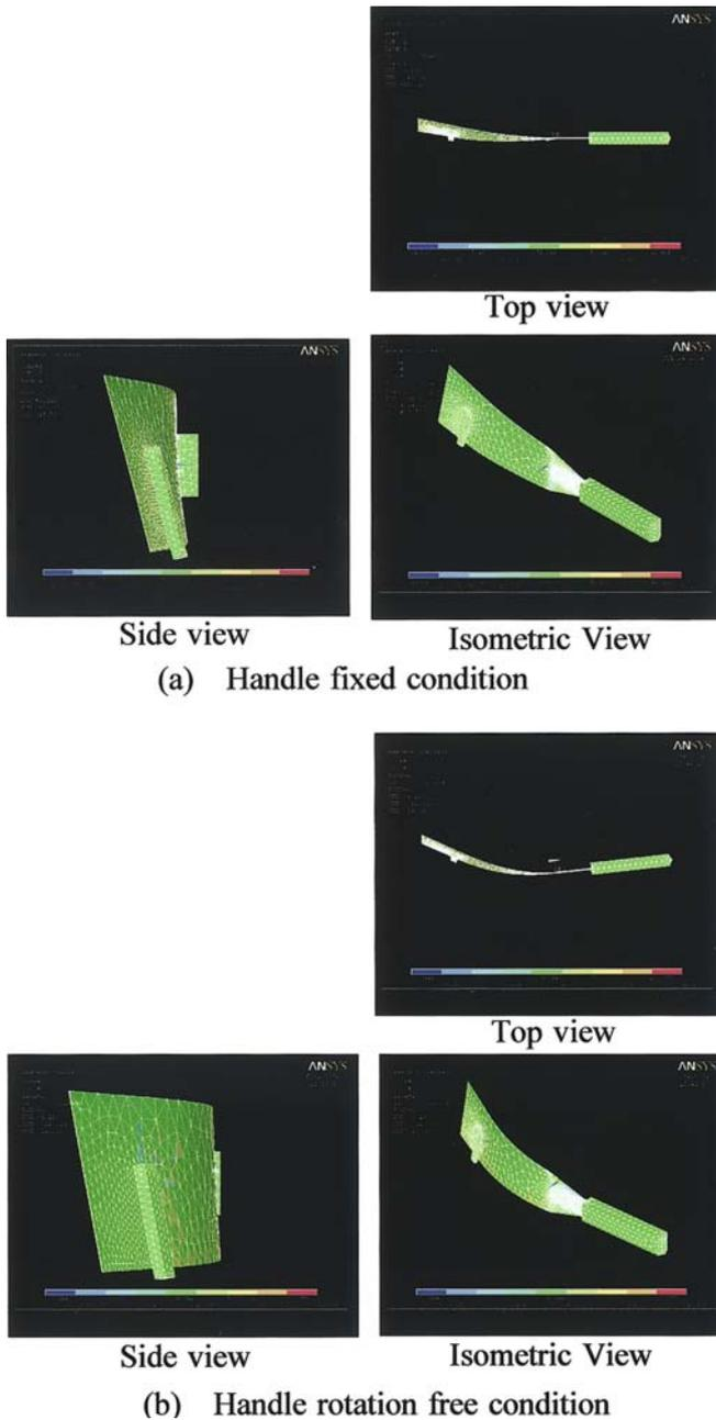
Fig. 8a,b. Deformation obtained by the finite element calculation for a fixed handle and b free handle conditions. Loading position: rectangular prism A, load values:  $F_H$  19N,  $F_V$  10N, Displacement magnification:  $\times 10$
