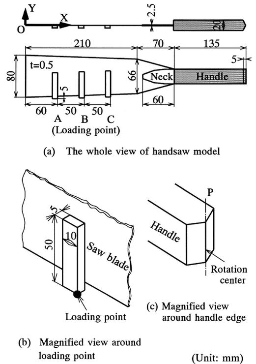
Fig. 4. Handsaw model for finite element model (FEM) calculation
