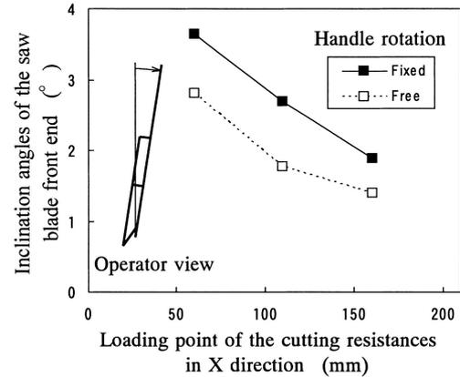
Fig. 6. Experimental inclination of the saw blade
