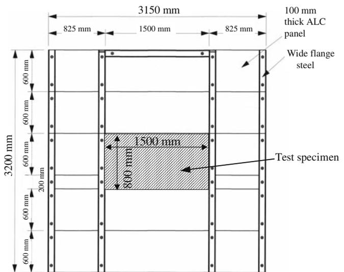
Fig. 1. Test specimen and specimen holder
