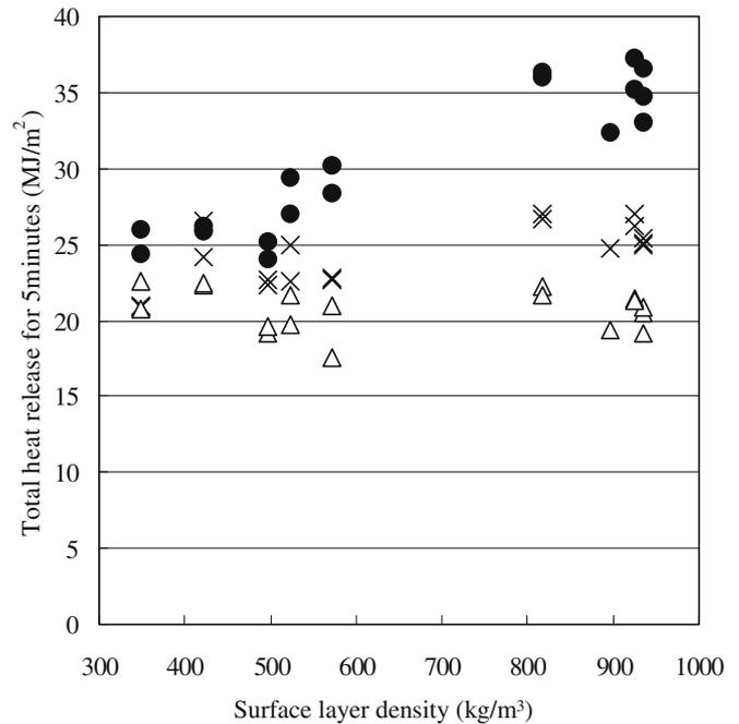
**Fig. 8.** Relationships between surface layer density and total heat release for 5 min. *Filled circles*, total heat release for 5 min from test start; *crosses*, total heat release for 5 min from 5 to 10min after test start; *open triangles*, total heat release for 5 min from 10 to 15min after test start
