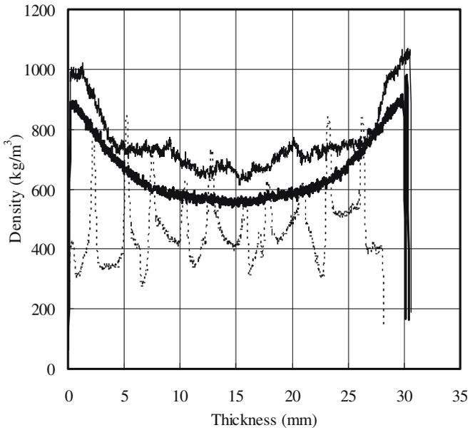
**Fig. 5.** Density profiles of plywood, particleboard (PB), and MDF. *Dashed line*, 28-mm-thick Japanese cedar plywood (JCPW 28mm); *thin solid line*, 30-mm-thick 18M-type particleboard (PB18M 30mm); *heavy solid line*, 30-mm-thick medium density fiberboard (MDF 30mm)
