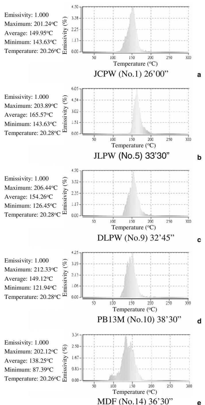
**Fig. 3a–e.** Temperature distribution of the unexposed side when the highest temperature reached 200°C. **a** JCPW; **b** JLPW; **c** DLPW; **d** PB13M; **e** MDF
