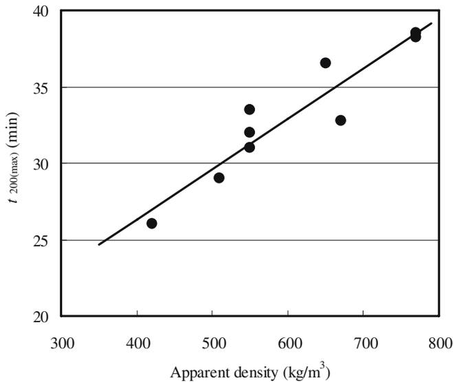
**Fig. 4.** Relationship between the apparent density of wood-based board and the time when the maximum temperature of the unexposed side reached 200°C [ $t_{200(max)}$ ] in the ISO 834-1 test. Filled circles, observed values; straight line, regression line
