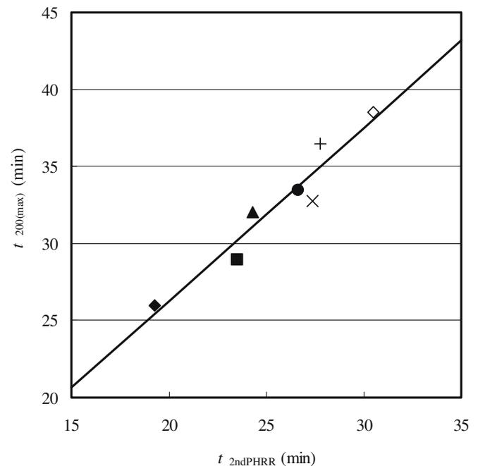
**Fig. 10.** Relationships between the time when the second peak of heat release rate appeared in the cone calorimeter test ( $t_{2ndPHRR}$ ) and the time when the maximum temperature of the unexposed side reached 200°C in the ISO 834-1 test [ $t_{200(max)}$ ]. The legends are the same as in Fig. 6
