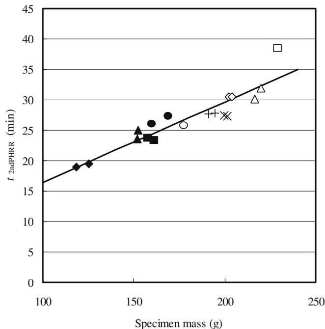
**Fig. 9.** Relationships between the specimen mass and the time when the second peak of heat release rate appeared. The legends are the same as in Fig. 6
