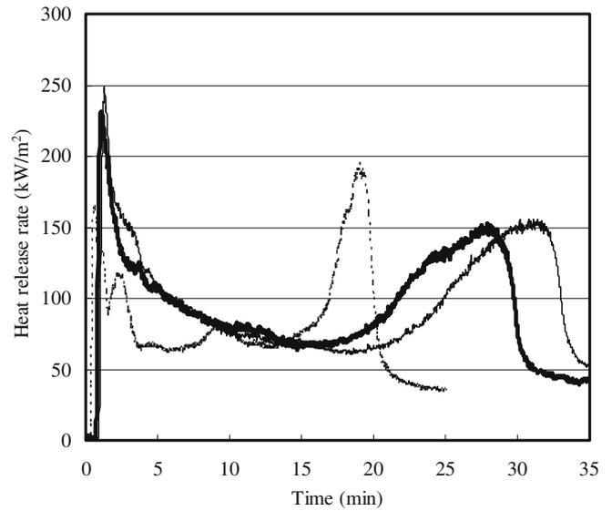
**Fig. 7.** Heat release rate curves of plywood, PB and MDF. *Dashed line*, JCPW 28mm; *thin solid line*, PB18M 30mm; *heavy solid line*, MDF 30mm
