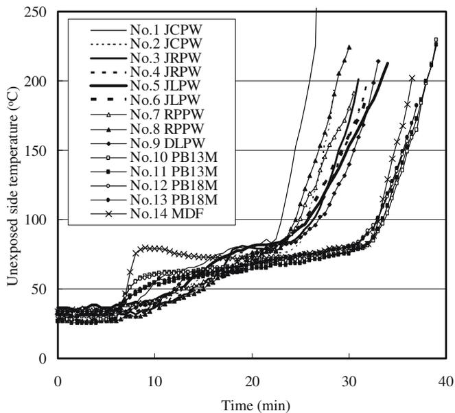
**Fig. 2.** Temperature of the unexposed side of the specimen. *JCPW*, Japanese cedar plywood; *JRPW*, Japanese red pine plywood; *JLPW*, Japanese larch plywood; *RPPW*, radiata pine plywood; *DLPW*, Dahurian larch plywood; *PB13M*, 13M-type particleboard; *PB18M*, 18M-type particleboard; *MDF*, medium density fiberboard
