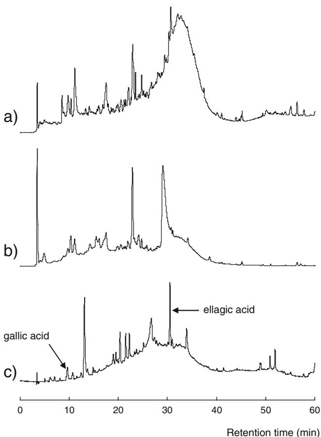
**Fig. 2a–c.** High performance liquid chromatography (HPLC) chromatograms of extracts from *Q. crispula* sapwood with detection at 280 nm. **a** Extracts from normal sapwood of *Q. crispula* (NS); **b** extracts from infected colored sapwood of *Q. crispula* (IS); **c** NS hydrolyzed with 3 N H<sub>2</sub>SO<sub>4</sub> at 110°C for 10 h
