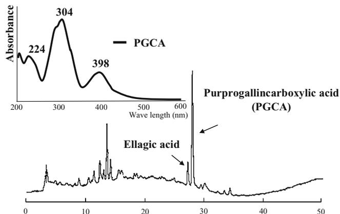
**Fig. 7.** HPLC chromatogram with detection at 400 nm of the water-soluble fraction of IS extracts. The ultraviolet absorption spectrum and the HPLC retention time of Compound 1 conformed with those of PGCA
