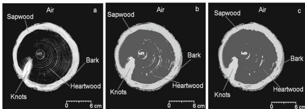
**Fig. 2a–c.** Examples of CT cross section images for the black spruce log. **a** Raw CT image, **b** image classified by the back propagation artificial neural network (BP ANN) classifier, and **c** classified image filtered using a  $5 \times 5$  pixel median filter
