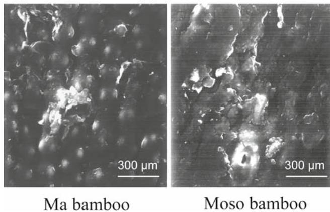
**Fig. 1.** Scanning electron micrographs of surface structure of ma bamboo (left) and moso bamboo (right) culms
