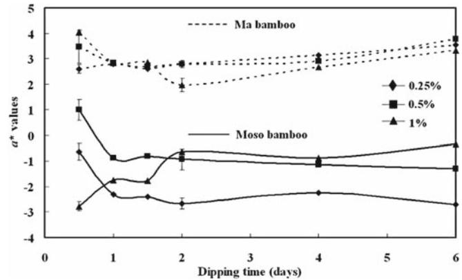
Fig. 3. Changes in  $a^*$  value of ma bamboo and moso bamboo treated with 0.25%, 0.5%, and 1% ACQ-B solution under ambient conditions for 6 days
