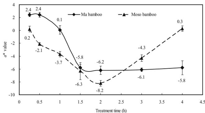
Fig. 2. Changes in  $a^*$  value for ma bamboo and moso bamboo culms after treatment with 0.25% ammoniacal copper quaternary compound-type B (ACQ-B) at 100°C for different times
