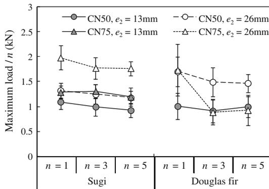
**Fig. 7** Maximum load divided by number of nails of nailed joints. Symbols and bars indicate mean value and standard deviation, respectively. *n* number of nails, *e*<sub>2</sub> edge distance
