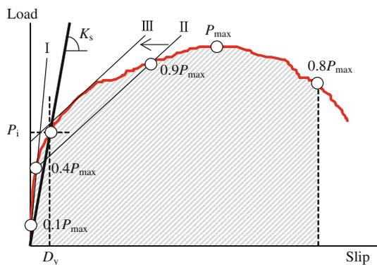
**Fig. 5** Method of evaluating shear performances of nailed joints.  $P_{max}$  maximum load,  $P_1$  load corresponding to the intersection of lines I and III,  $D_y$  yield slip,  $K_s$  initial stiffness
