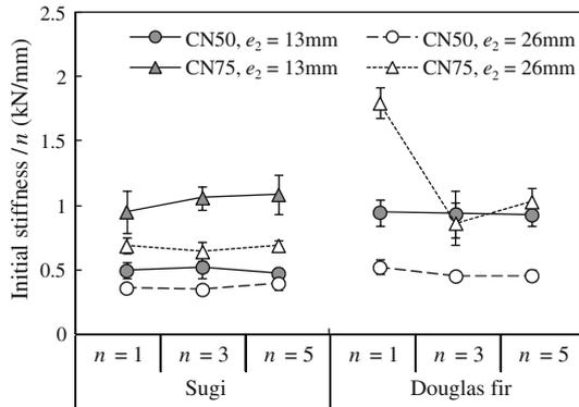
**Fig. 6** Initial stiffness divided by number of nails of nailed joints. Symbols and bars indicate mean value and standard deviation, respectively. *n* number of nails, *e*<sub>2</sub> edge distance
