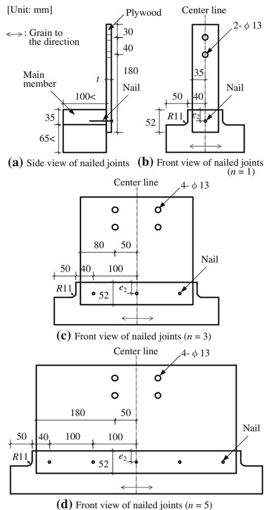
**Fig. 1** Configuration of nailed joint specimen.  $e_2$  edge distance of the main member: 13 or 26 mm,  $t$  thickness of plywood: 12 or 24 mm,  $n$  number of nails
