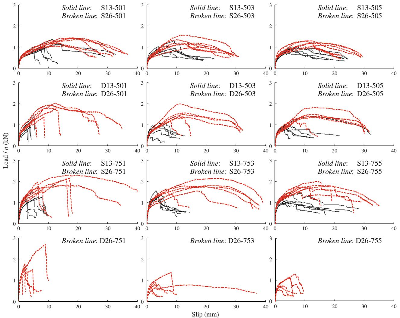
**Fig. 4** Relations between load divided by number of nails and slip of nailed joints. For the symbols, see Table 1
