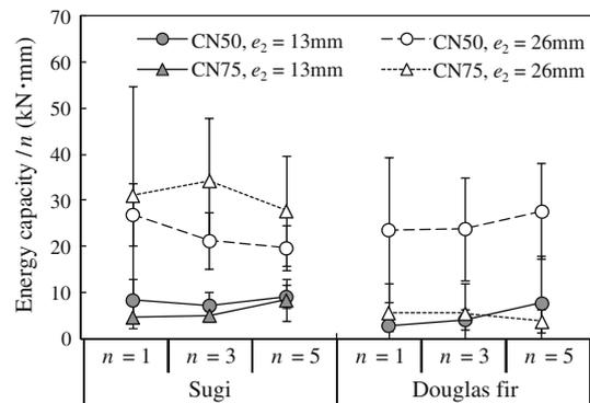
**Fig. 8** Energy capacity divided by number of nails of nailed joints. Symbols and bars indicate mean value and standard deviation, respectively. *n* number of nails, *e*<sub>2</sub> edge distance
