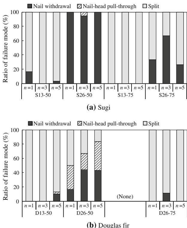
**Fig. 3** Failure modes of nailed joints loaded perpendicular to the grain. For the symbols, see Table 1. **a** Nailed joints with Sugi as the main member. **b** Nailed joints with Douglas fir as the main member.  $n$  number of nails,  $e_2$  edge distance
