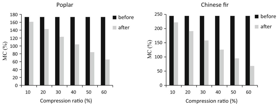
**Fig. 2** Moisture content (MC) before and after compression showing an increased difference with the increase of compression ratio
