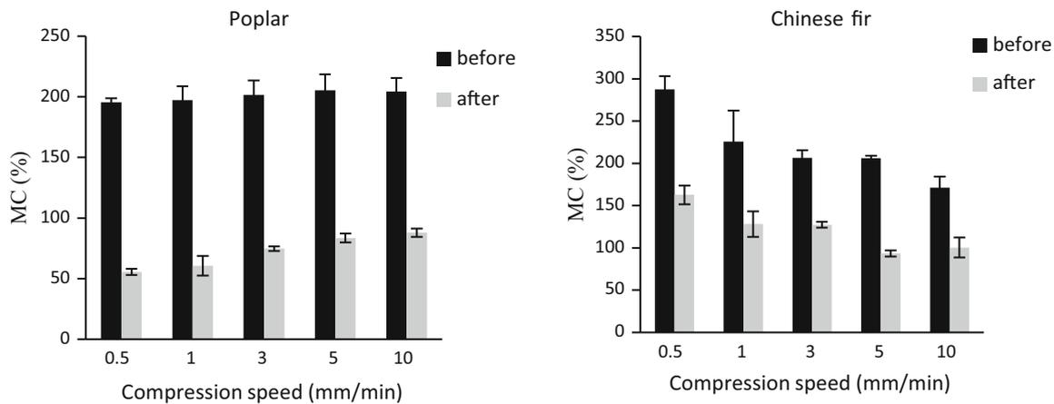
**Fig. 6** Moisture content (MC) before and after compression at the different compression speed
