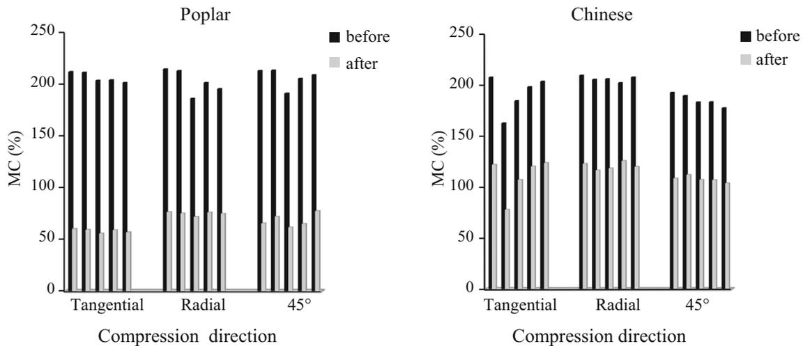
**Fig. 5** Moisture content (MC) before and after compression showing a big difference in 3 directions compression
