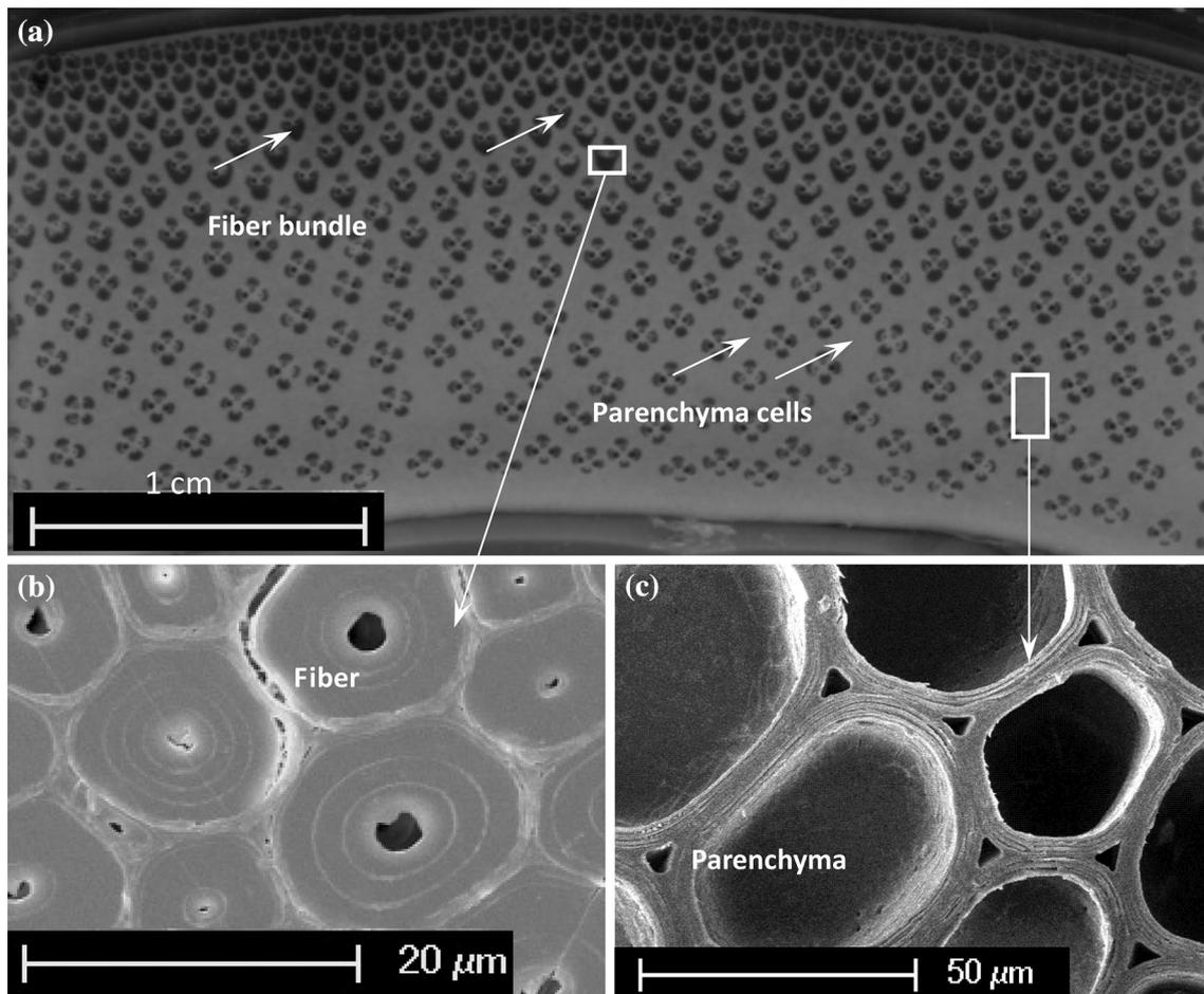
**Fig. 8** SEM images showing the morphologies of bamboo transverse section (a), bamboo fibers (b) and parenchyma cells (c)
