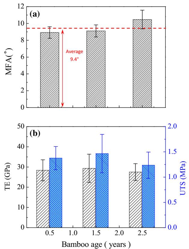
**Fig. 5** Microfibril angle and mechanical properties of single bamboo fibers. **a** MFA of Moso bamboo; **b** histogram of TE and UTS of single bamboo fibers. *MFA* microfibrillar angle, *TE* longitudinal tensile modulus, *UTS* ultimate tensile strength
