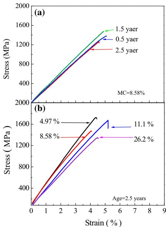
**Fig. 4** The typical stress–strain curves of single bamboo fibers with different ages (a) and MC (b) tensioned in axial direction
