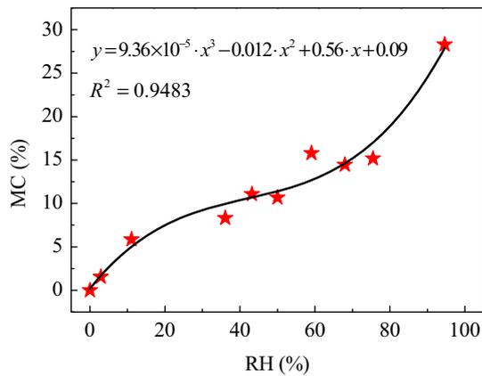
**Fig. 3** The moisture sorption isotherms of bamboo fibers. *MC* moisture content, *RH* relative humidity
