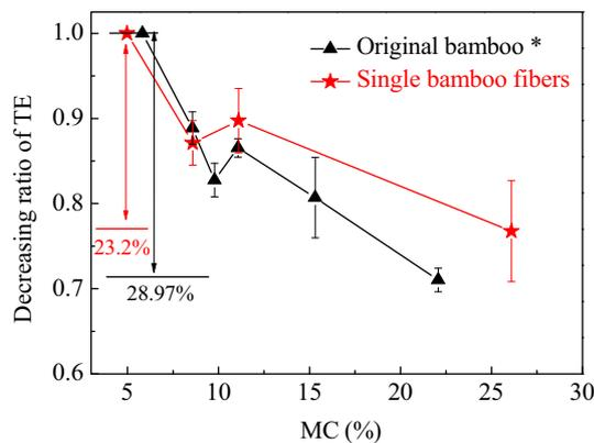
**Fig. 7** The decreasing ratio of TE of single bamboo fiber and solid bamboo from 4.97 to 26.2 %. Asterisk TE and MC of solid bamboo quoted from Jiang et al. [34]. TE longitudinal tensile modulus, MC moisture content
