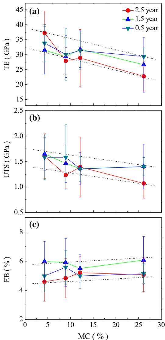
**Fig. 6** The influence of MC on longitudinal tensile properties of single bamboo fibers. *TE* longitudinal tensile modulus, *UTS* ultimate tensile strength, *EB* elongation at break, *MC* moisture content
