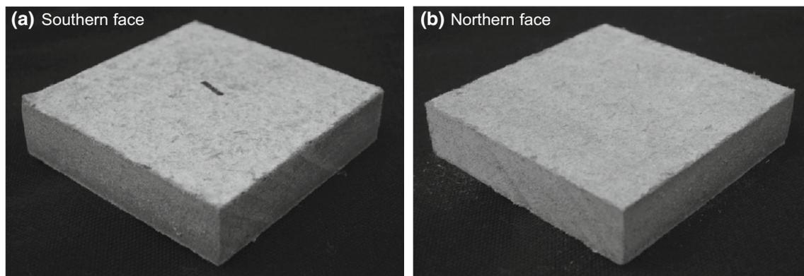
**Fig. 7** The surface of methylene diphenyl diisocyanate resin-bonded medium-density fiberboard (MDF) subjected to outdoor exposure after 5 years at site 4. The site no. is described in Table 1
