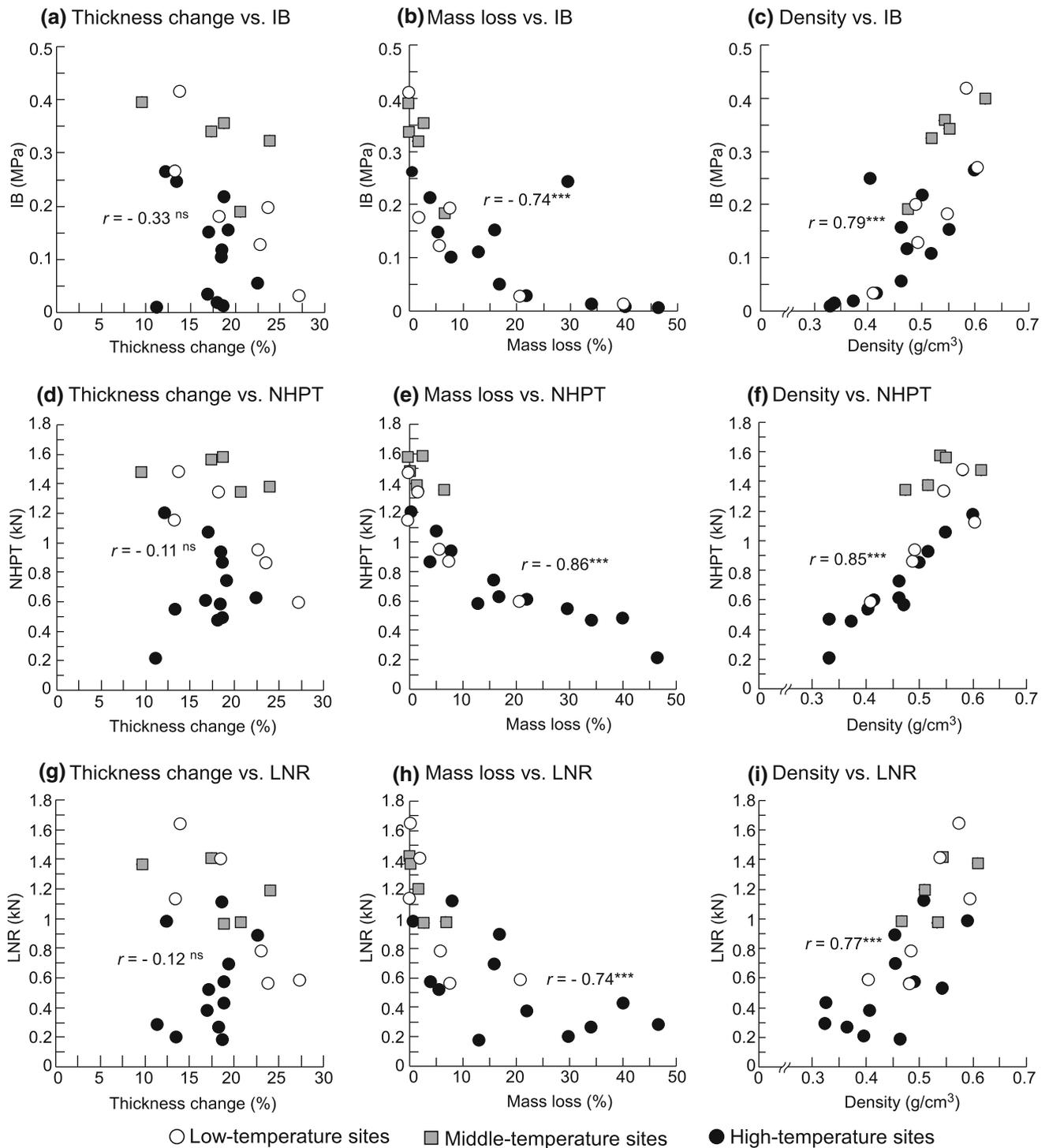
**Fig. 10** Relationships among the thickness change, mass loss, density, and mean board strength [internal bond strength (IB), nail-head pull-through strength (NHPT), and lateral nail resistance (LNR)] of oriented strand board (OSB) manufactured from aspen subjected to
