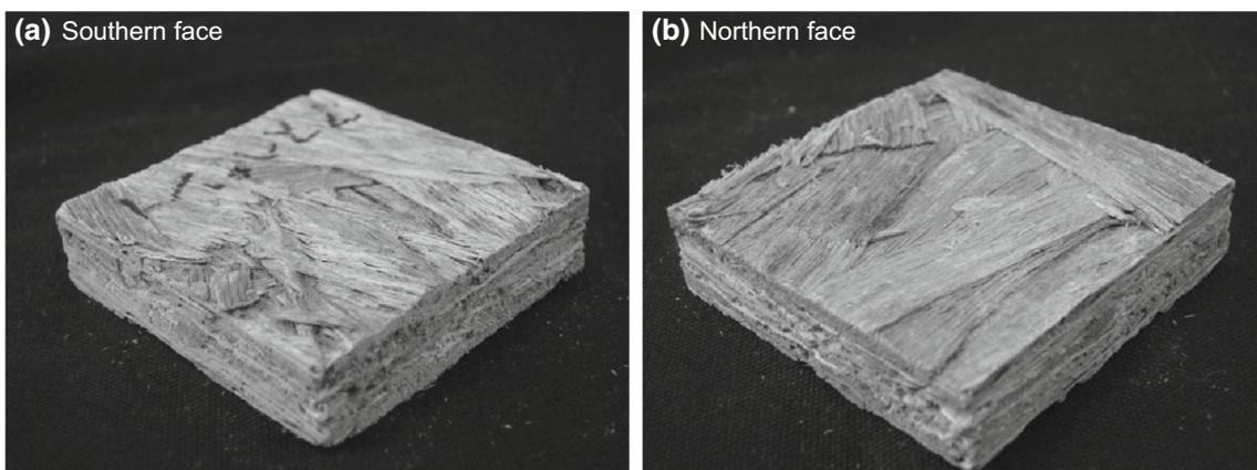
**Fig. 6** The surface of oriented strand board (OSB) manufactured from aspen subjected to outdoor exposure after 5 years at site 4. The site no. is described in Table 1
