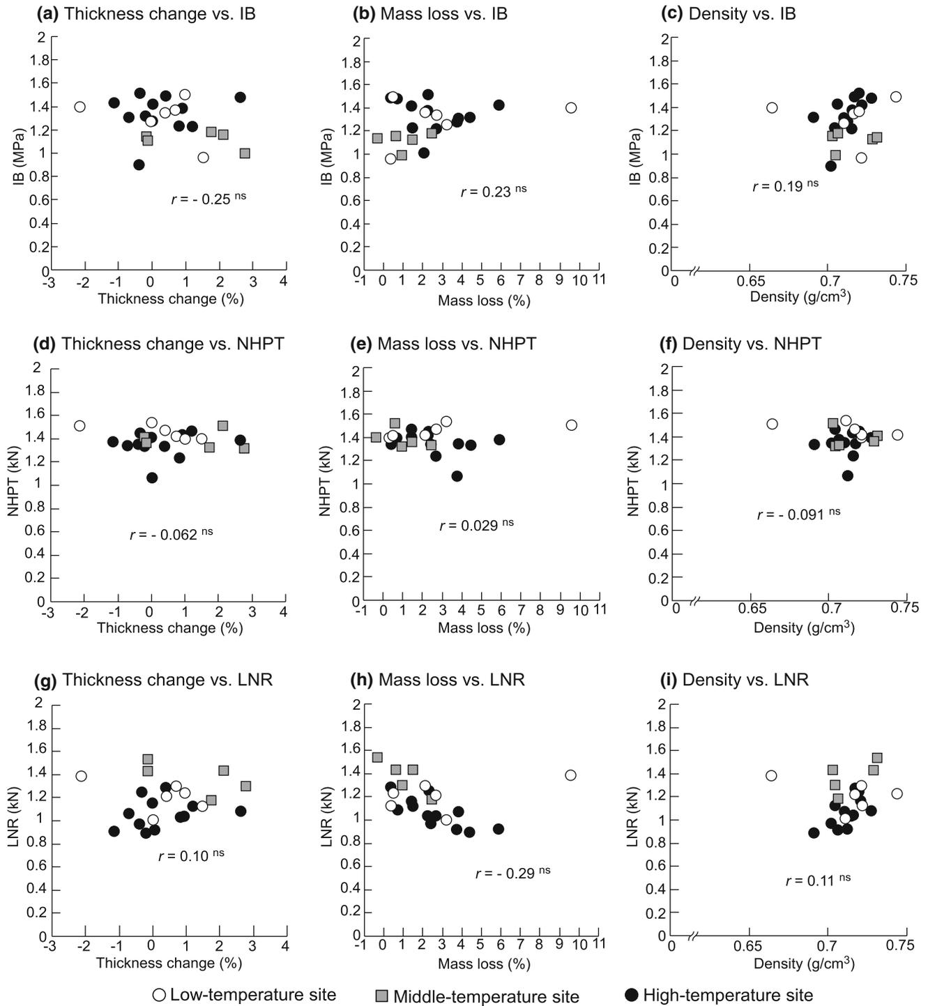
**Fig. 11** Relationships among the thickness change, mass loss, density, and mean board strength [internal bond strength (IB), nail-head pull-through strength (NHPT), and lateral nail resistance (LNR)] of methylene diphenyl diisocyanate resin-bonded medium-density
