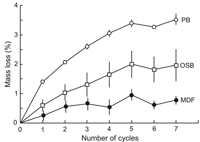
**Fig. 4** Relationships between cycle and mean mass loss for phenol–formaldehyde resin-bonded particleboard (PB), oriented strand board (OSB) manufactured from aspen, and methylene diphenyl diisocyanate resin-bonded medium-density fiberboard (MDF). Error bars standard deviations. The specimens were immersed in water at 70 °C for 6 h followed by drying at 105 °C for 16 h (one cycle) and repeating the process for seven cycles
