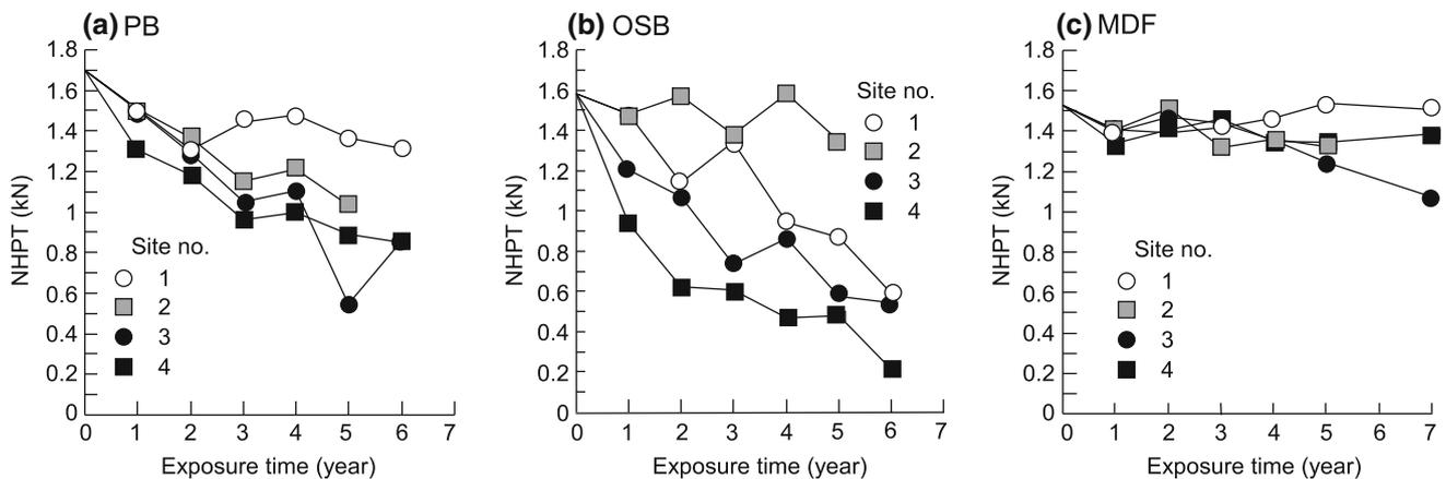
**Fig. 2** Relationships between exposure time and mean nail-head pull-through strength (NHPT) at the four sites for **a** phenol–formaldehyde resin-bonded particleboard (PB), **b** oriented strand board (OSB) manufactured from aspen, and **c** methylene diphenyl
