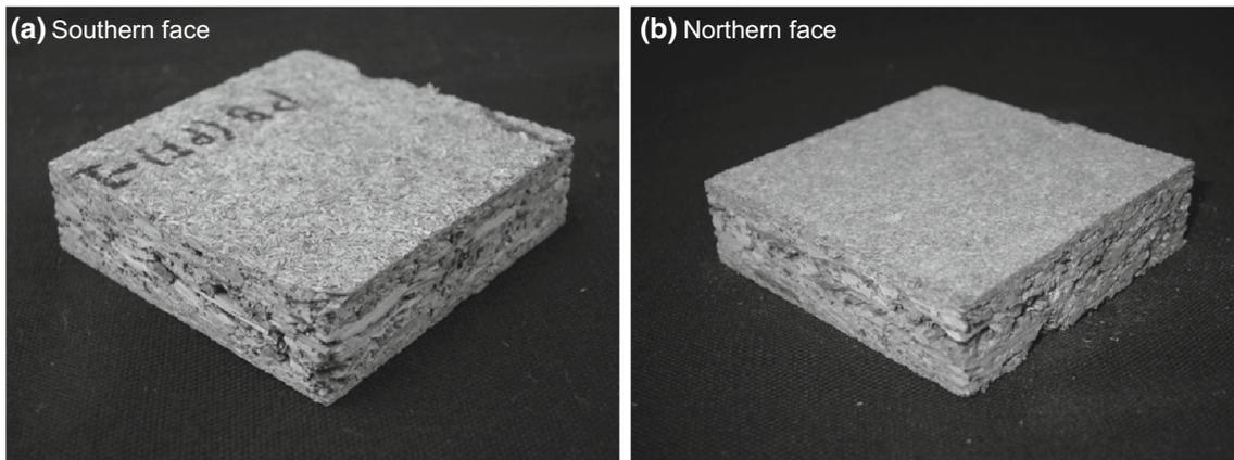
**Fig. 5** The surface of phenol-formaldehyde resin-bonded particleboard (PB) subjected to outdoor exposure after 5 years at site 4. The site no. is described in Table 1
