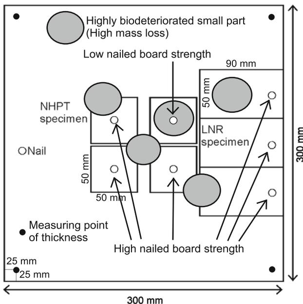
**Fig. 1** Trimming of NHPT specimens measuring 50 × 50 mm and LNR specimens measuring 90 × 50 mm and locally biodeteriorated specimen measuring 300 × 300 mm subjected to outdoor exposure. *NHPT* nail-head pull-through strength, *LNR* lateral nail resistance strength
