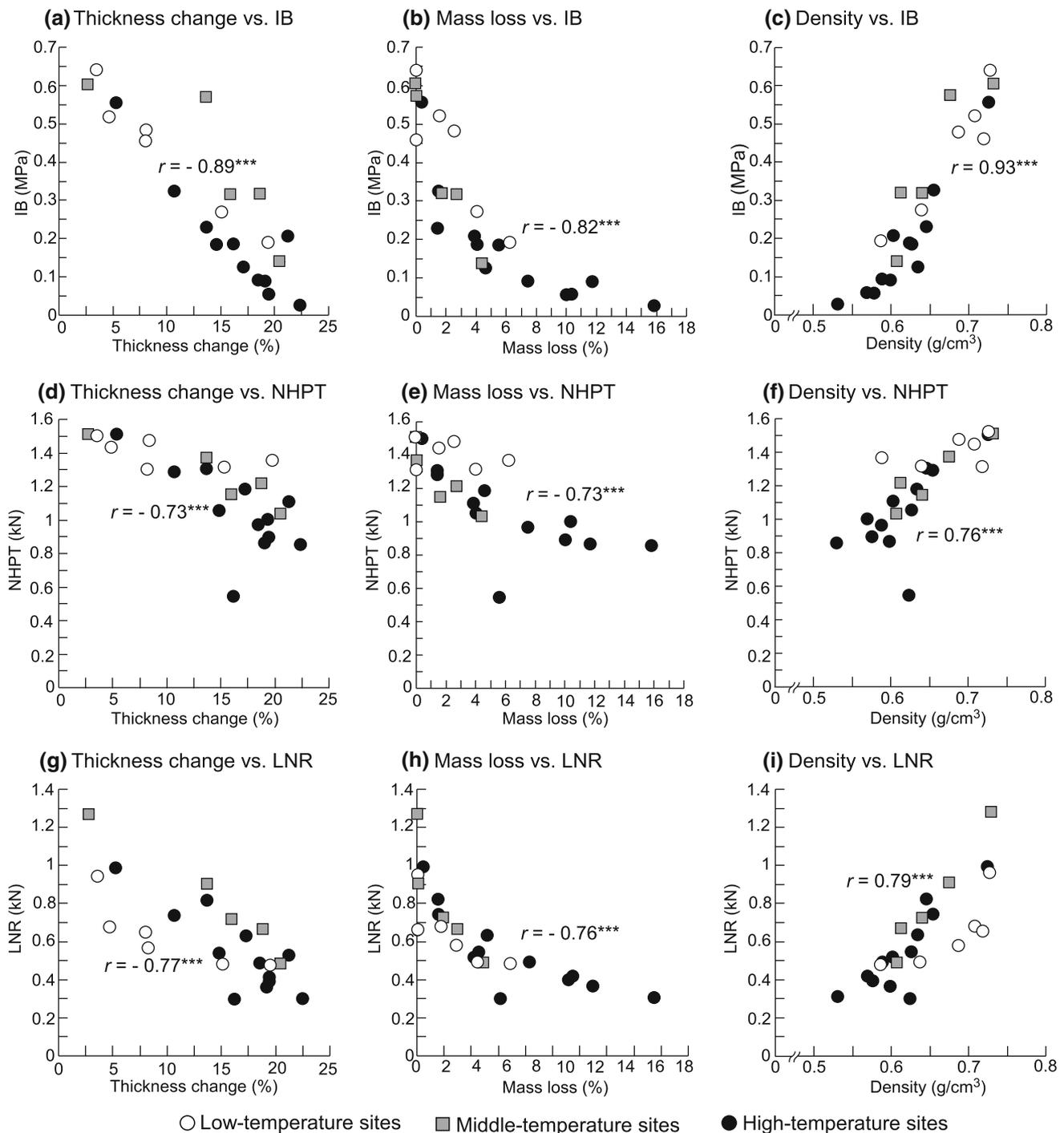
**Fig. 9** Relationships among the thickness change, mass loss, density, and mean board strength (internal bond strength (IB), nail-head pull-through strength (NHPT), and lateral nail resistance (LNR)) of phenol-formaldehyde resin-bonded particleboard (PB) subjected to
