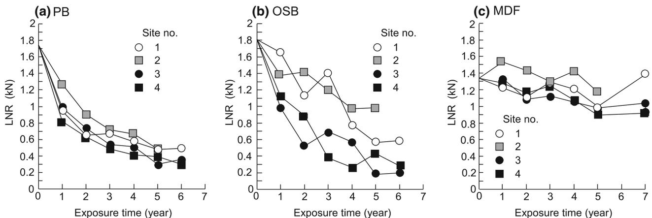
**Fig. 3** Relationships between exposure time and mean lateral nail resistance strength (LNR) at the four sites for **a** phenol–formaldehyde resin-bonded particleboard (PB), **b** oriented strand board (OSB) manufactured from aspen, and **c** methylene diphenyl diisocyanate
