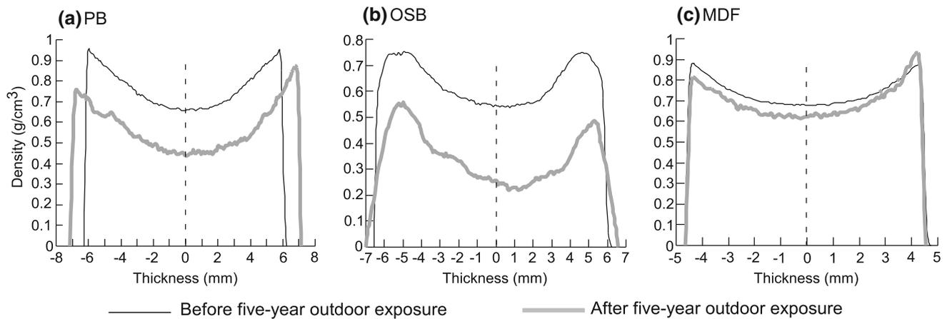
**Fig. 8** Density profiles of phenol-formaldehyde resin-bonded particleboard (PB), oriented strand board (OSB) manufactured from aspen, and methylene diphenyl diisocyanate resin-bonded medium-density
