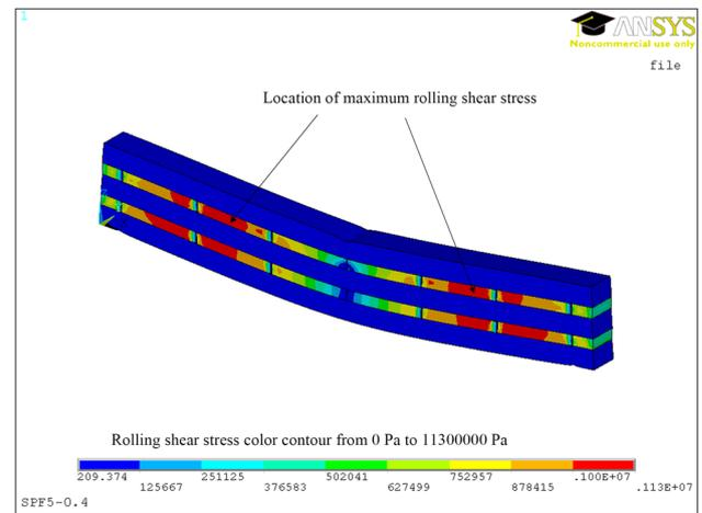
**Fig. 13** Rolling shear stress distribution in 5-layer CLT specimen under 12.51 kN load (stress in Pa)
