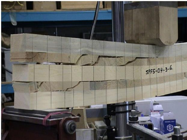
**Fig. 7** Failure mode in the ramp loading test
