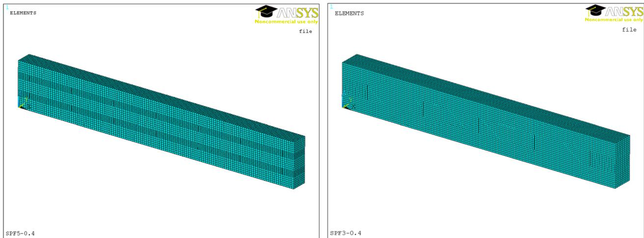
**Fig. 11** Finite element modeling of the CLT beam test specimens
