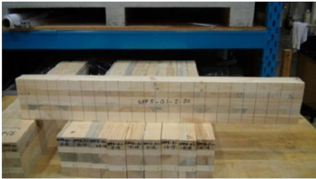
**Fig. 4** CLT beam specimens
