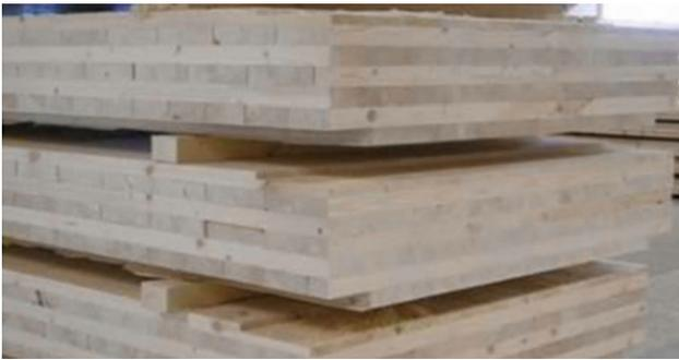
**Fig. 1** Layering of cross laminated timber (CLT)
