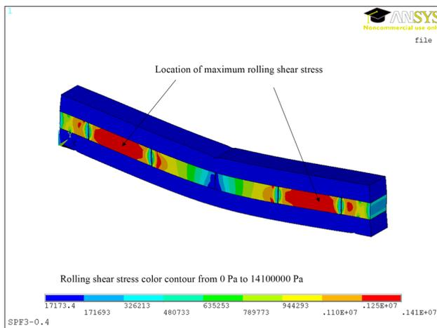
**Fig. 12** Rolling shear stress distribution in 3-layer CLT specimen under 12.51 kN load (stress in Pa)
