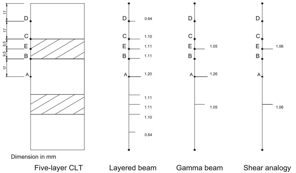
**Fig. 10** Shear stress evaluated in the cross section of the CLT beam (in  $N/mm^2$  under 19.39 kN centre-point load)
