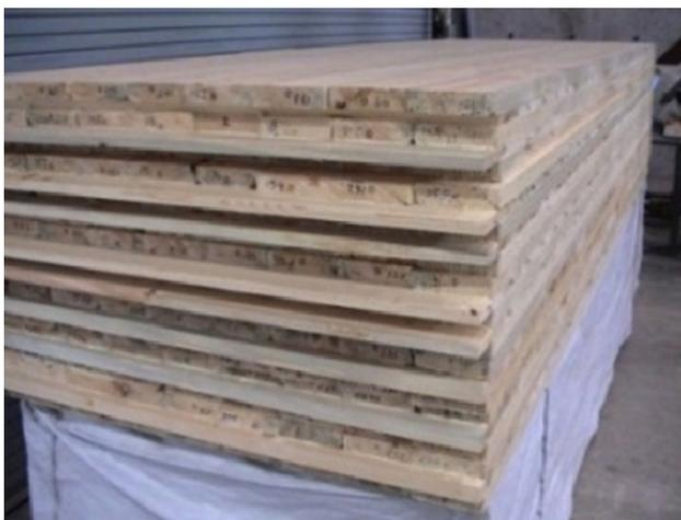
**Fig. 3** CLT panels
