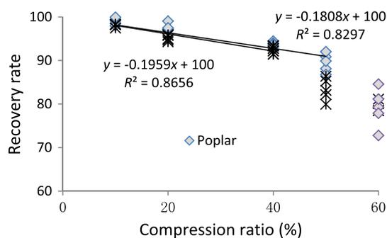
**Fig. 2** Linear relations between the recovery rate and compression ratio when the compression ratio  $\leq 50$  % (Poplar) or  $\leq 40$  % (Chinese fir)
