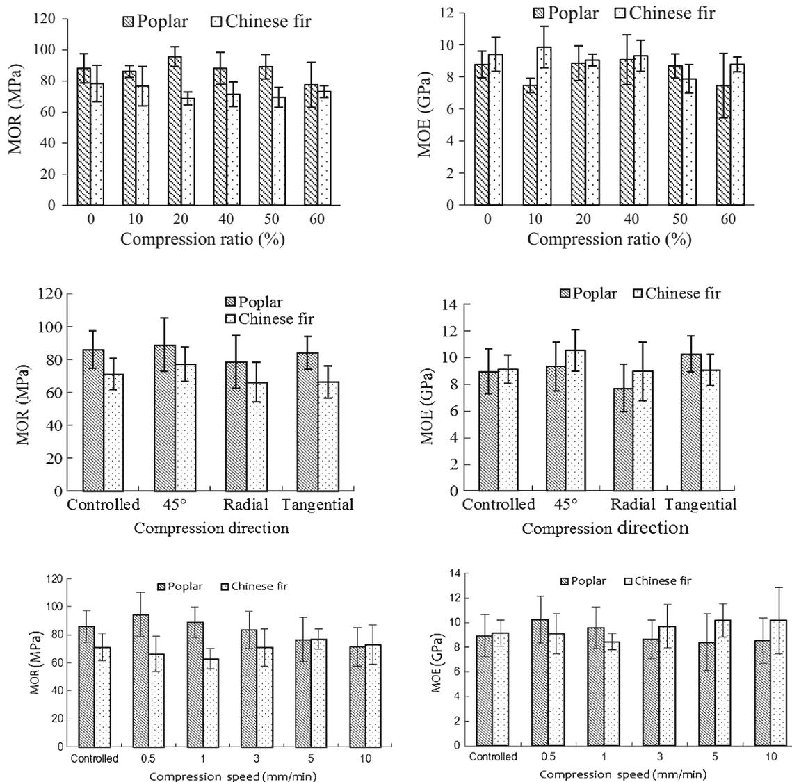
**Fig. 3** Mechanical properties in static bending showing that they were well retained after the pre-treatment by compression at different compression ratio, different compression direction and different compression speed. *MOR* modulus of rupture, *MOE* modulus of elasticity
