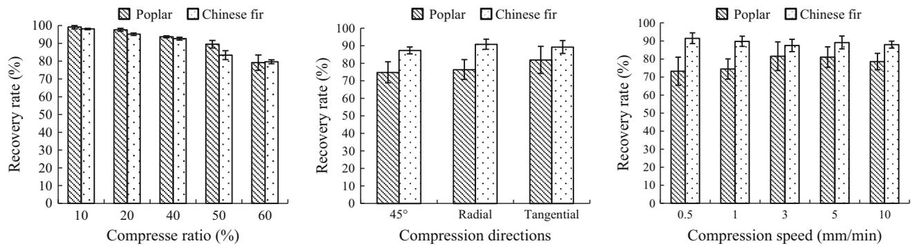
**Fig. 1** Wood recovery rate at different compression ratio, compression direction and compression speed
