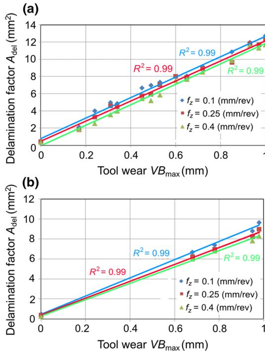
**Fig. 10** Dependence of the delamination factor  $A_{del}$  vs. high-speed steel tool wear for cutting speeds:  $v_c = 4.40$  m/s (a) and  $v_c = 13.19$  m/s (b)
