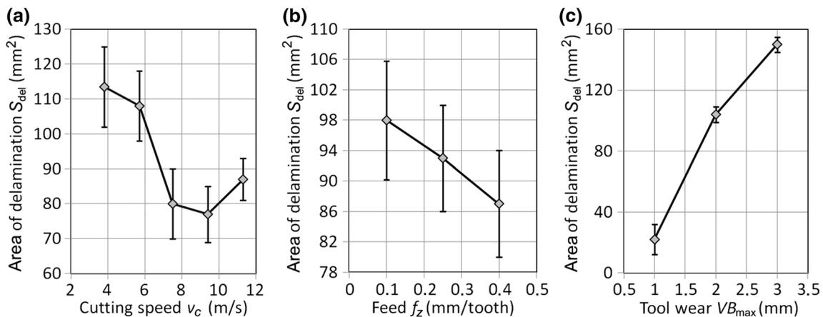
**Fig. 11** Influence of cutting speed  $v_c$  (a) and feed  $f_z$  (b), and tool wear (c) on the value of area of delamination for high-speed steel tool
