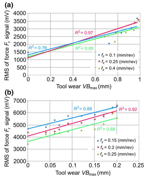
**Fig. 9** Dependence of the root-mean-square (RMS) of force  $F_y$  signal vs. tool wear at  $v_c = 13.9$  m/s for high-speed steel tool (a) and cemented carbide tool (b)
