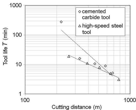
**Fig. 4** Influence of cutting speed on the tool life
