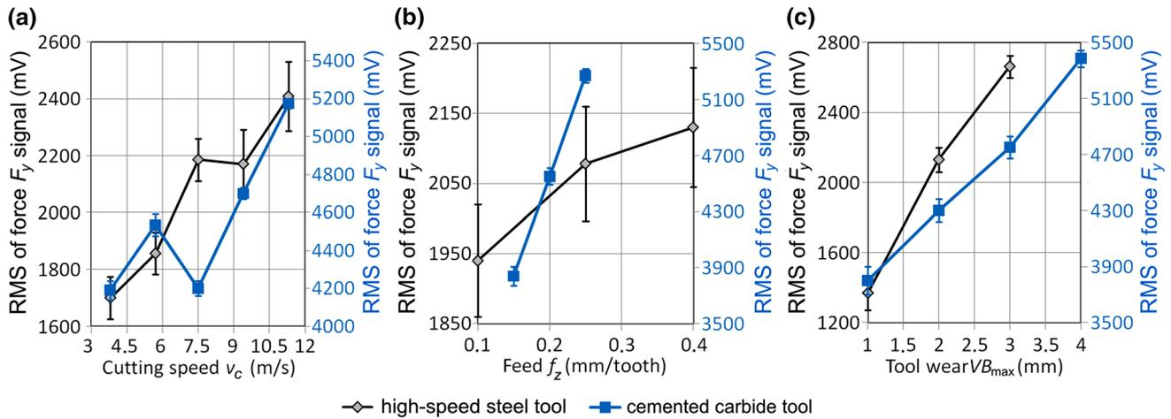
**Fig. 7** Effect of cutting parameters  $v_c$  (a) and feed  $f_z$  (b), and tool wear (c) on the value of root-mean-square (RMS) of signals of force  $F_y$
