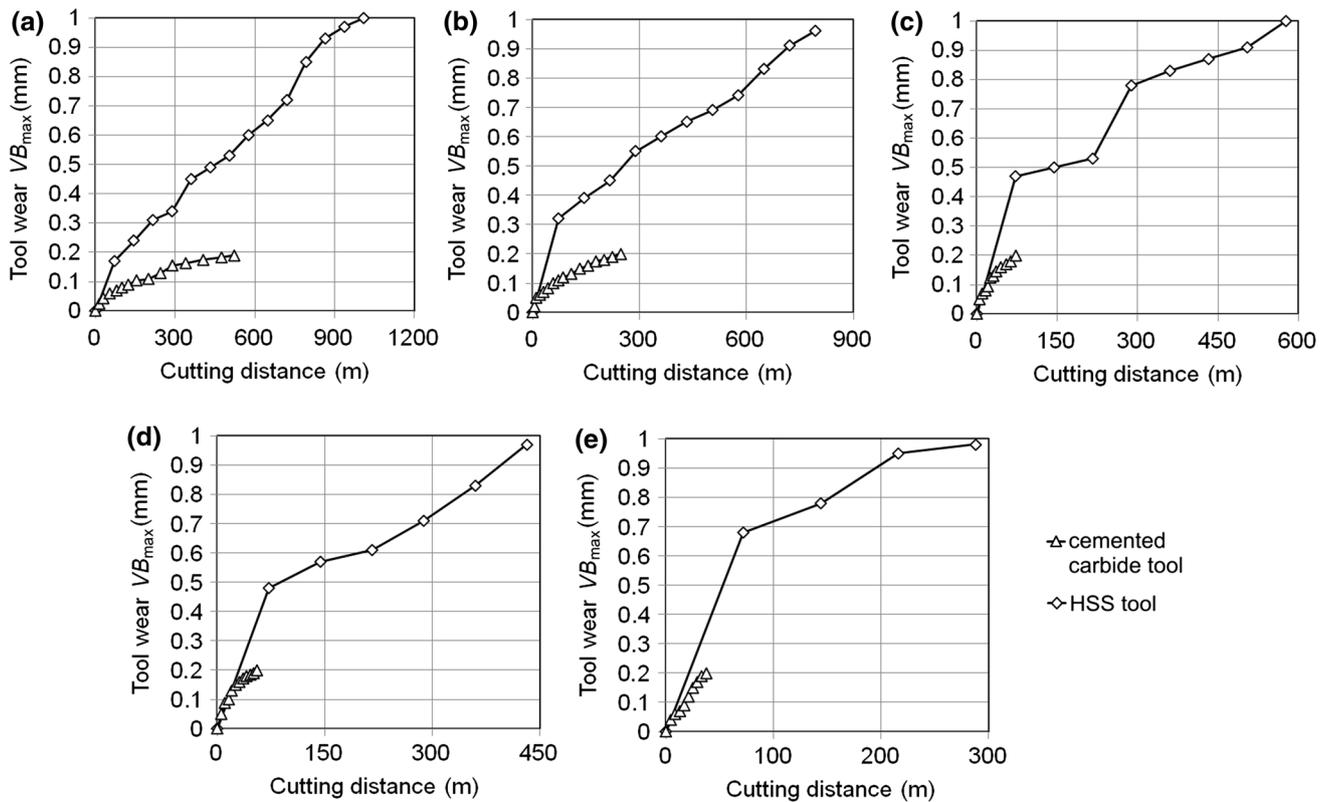
**Fig. 5** Variation of tool wear as a function of cutting distance: **a**  $n = 6000$  rev/min, **b**  $n = 9000$  rev/min, **c**  $n = 12000$  rev/min, **d**  $n = 15000$  rev/min, **e**  $n = 18000$  rev/min;  $f_z = 0.25$  mm/tooth
