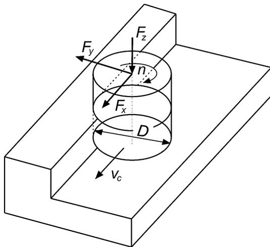
**Fig. 2** Distribution of force components in the milling process
