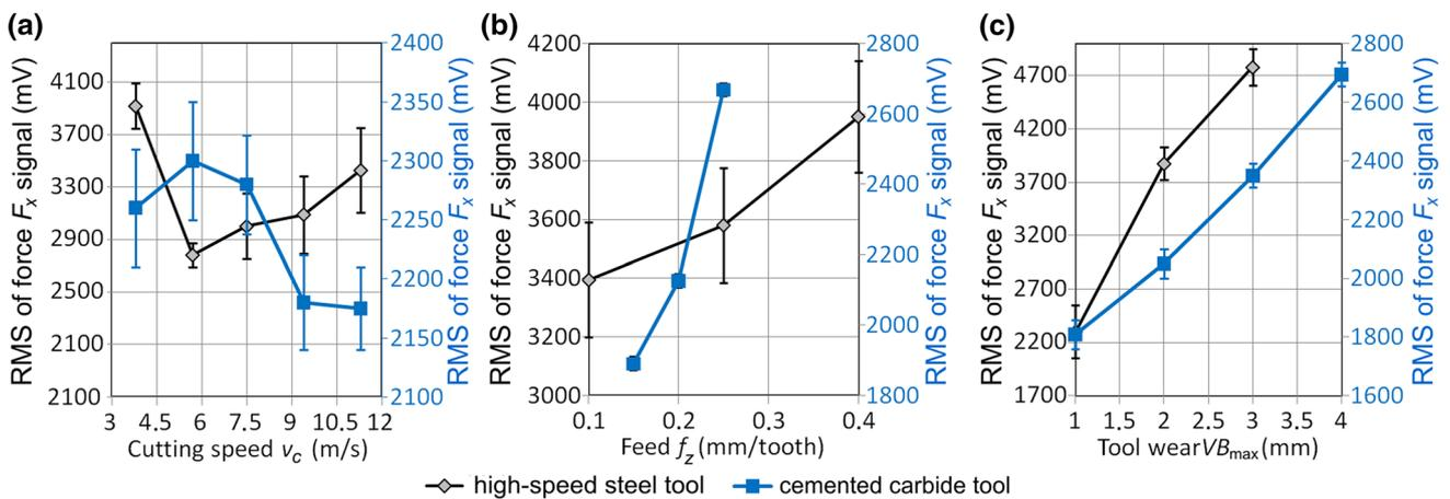
**Fig. 6** Effect of cutting parameters  $v_c$  (a) and feed  $f_z$  (b), and tool wear (c) on the value of root-mean-square (RMS) of signals of force  $F_x$
