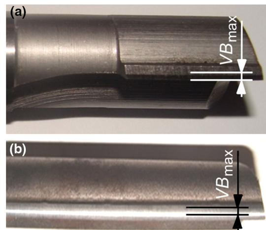
**Fig. 1** Milling tools: **a** high-speed steel bit and **b** cemented carbide shank-type bit
