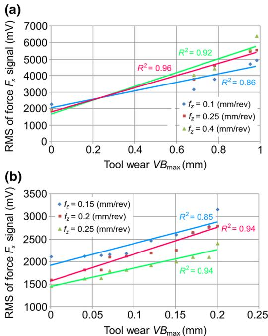
**Fig. 8** Dependence of the root-mean-square (RMS) of force  $F_x$  signal vs. tool wear at  $v_c = 13.9$  m/s for high-speed steel tool (a) and cemented carbide tool (b)
