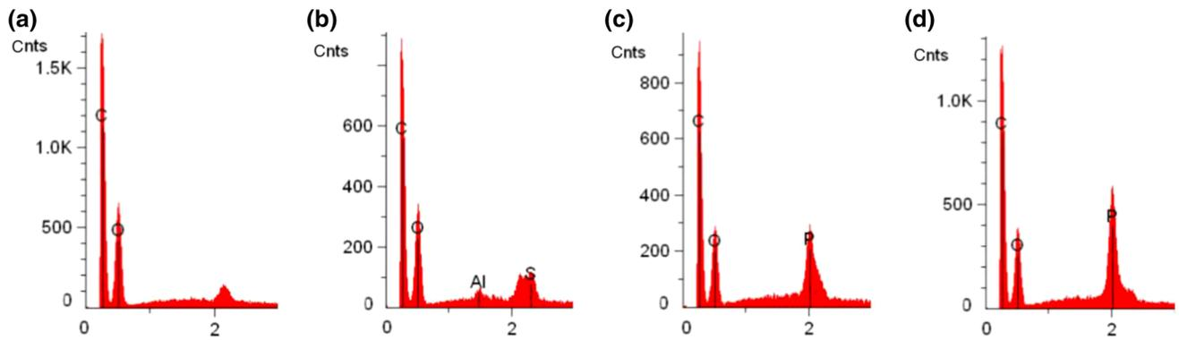
**Fig. 6** Electron dispersive X-ray (EDX) spectra of **a** wood, **b** wood with lactide, **c** wood with resorcinol *bis*(diphenyl phosphate) (RDP), and **d** wood with lactide and resorcinol *bis*(diphenyl phosphate) (RDP)
