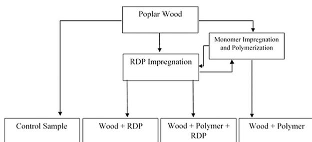
**Fig. 3** Outline of procedures used to manufacture the wood-plastic combination (WPC) and the subsequent four materials formed
