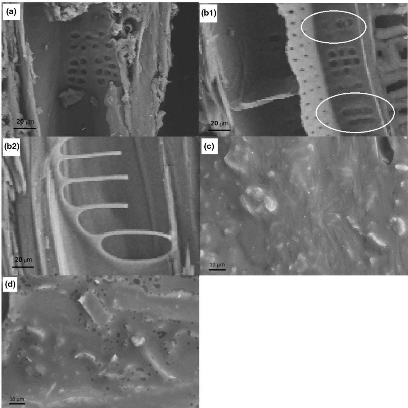
**Fig. 5** Scanning electron microscope (SEM) image of **a** wood, **b1**, **b2** wood with lactide, **c** wood with resorcinol *bis*(diphenyl phosphate) (RDP), and **d** wood with lactide and resorcinol *bis*(diphenyl phosphate) (RDP)
