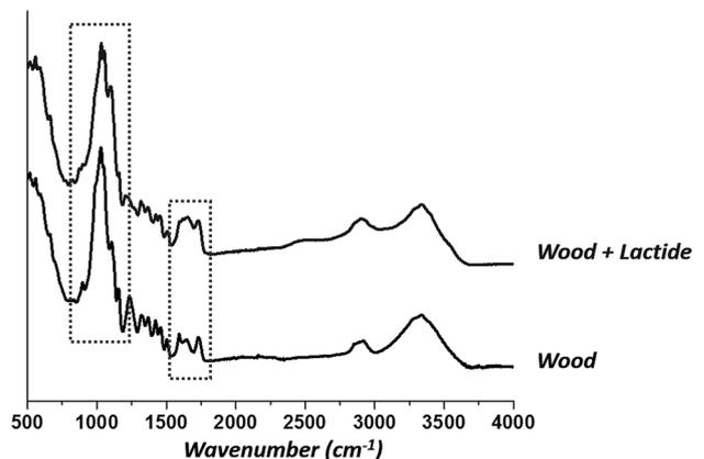
**Fig. 8** Fourier transform infrared spectroscopy (FTIR) spectrum of the wood/lactide composite compared to the control wood spectrum
