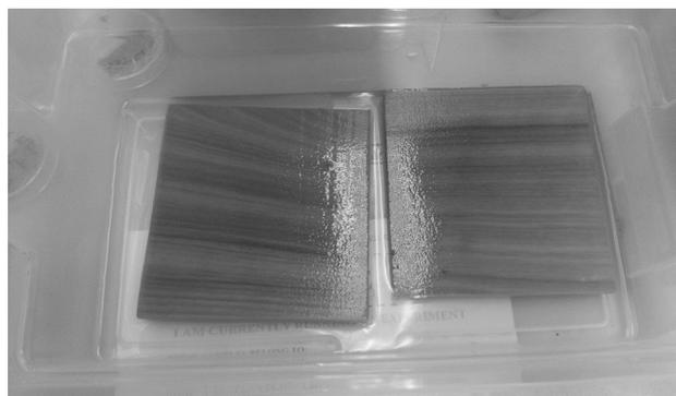
**Fig. 2** Wood samples soaked in monomer solution preceding vacuum impregnation and heat polymerization
