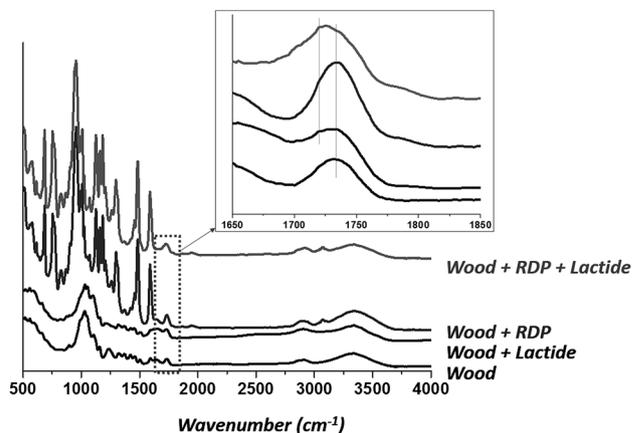
**Fig. 9** Fourier transform infrared spectroscopy (FTIR) spectra of the four wood and wood-plastic combination (WPC) samples
