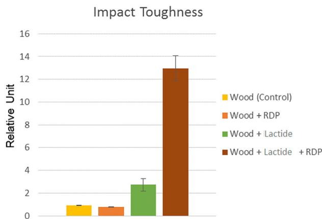
**Fig. 4** Impact toughness values of control wood, wood treated with resorcinol *bis*(diphenyl phosphate)(RDP), and the two wood-plastic combination (WPC) samples where the value for the control sample was  $I = 42.5 \pm 5.0 \text{ kJ/m}^2$
