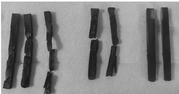
**Fig. 7** Treated samples after conducting the UL-94 Flame Test, from *left*: 3 wood/PLA samples, 2 wood/resorcinol *bis*(diphenyl phosphate) (RDP) samples, and 2 wood/resorcinol *bis*(diphenyl phosphate) (RDP)/PLA samples. The minor discoloration at the top ends of the wood/resorcinol *bis*(diphenyl phosphate)(RDP)/PLA composites resulted from polymerization; it is unrelated to the flame test
