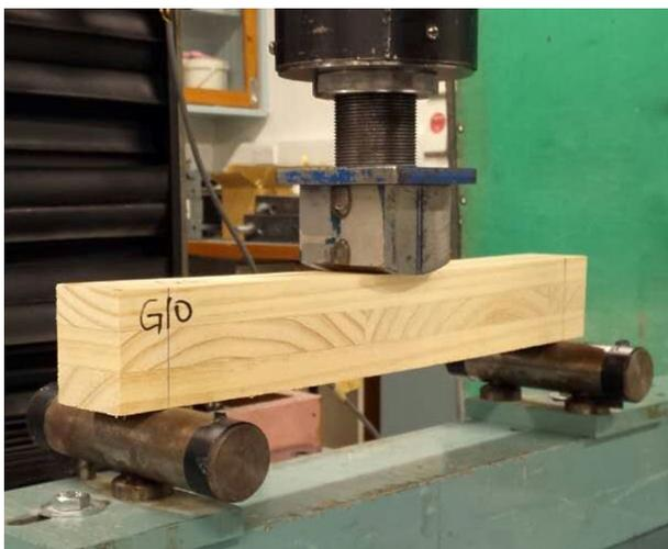
**Fig. 2** Short-span bending test setup
