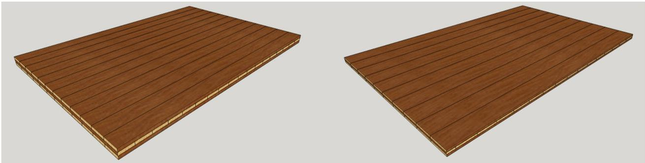
**Fig. 1** CLT plates with 35/35/35 layup and 20/20/20 layup
