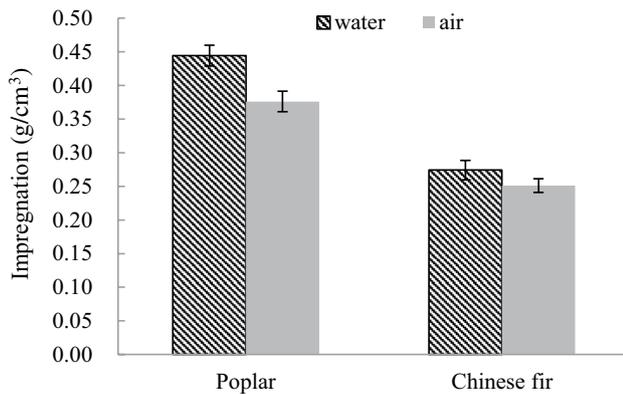
**Fig. 4** Impregnation comparison of wood after pre-treatment by compression and unloaded in water and in air
