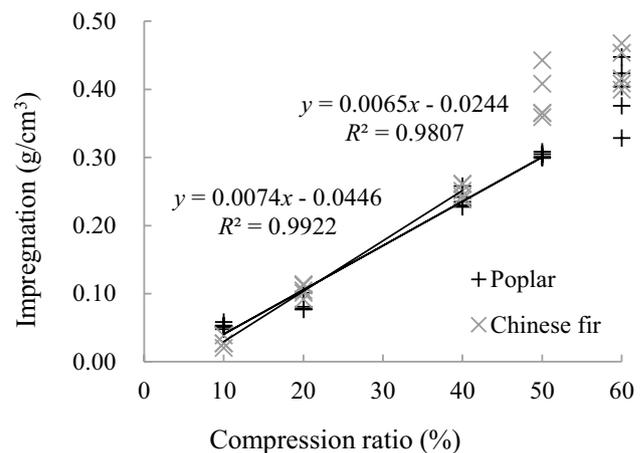
**Fig. 2** Linear relations between the impregnation and the compression ratio when the compression ratio  $\leq 50\%$  (poplar) or  $\leq 40\%$  (Chinese fir)
