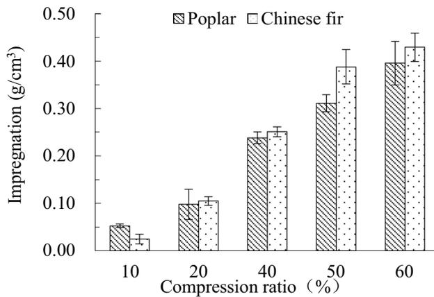
**Fig. 1** Impregnation of specimens after the pre-treatment by compression at different compression ratio
