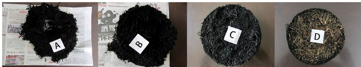
Fig. 3 The used wood fiber elements. A is the nearest to the inlet of the DPF, B close to A , C close to B , and D is the nearest to the outlet of the DPF
