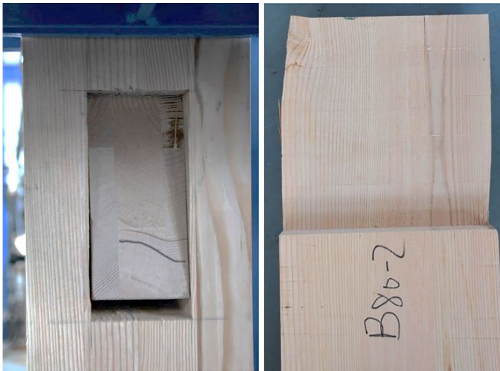
Fig. 5 Failure mode of the unreinforced mortise and tenon joint (specimen C1-2)
