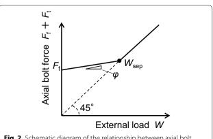
**Fig. 2** Schematic diagram of the relationship between axial bolt force and external load
