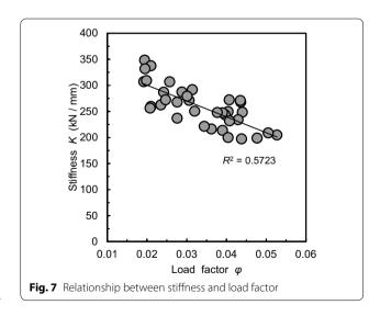
to the member end (L). Therefore, we can deduce that the spring constant and load factor varied in response to changes in stress distribution to  $F_{\rm f}$  in the L = 100, 130,
