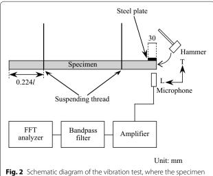
Fig. 2 Schematic diagram of the vibration test, where the specimer is suspended by two threads
