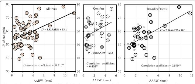
**Fig. 10** Correlation diagrams between AARW and  $L^*$  of end grain of each test piece. Each test piece number is shown as in Tables 1 and 3. Significance test results of correlation coefficient \*\*p < 0.01
