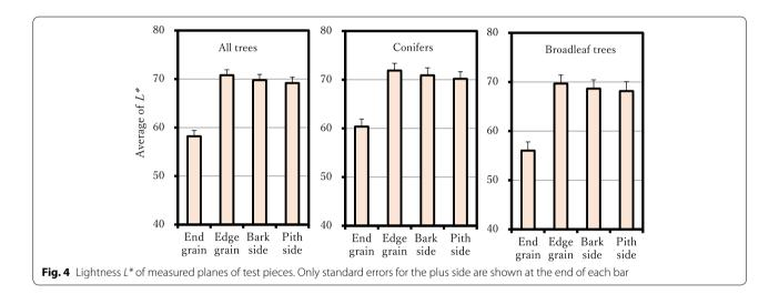
For broadleaf trees, there are significant differences of 1% between the end grain and each of the other planes for both  $a^*$  and  $b^*$ .
