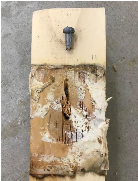
Fig. 8 Ruptured screw and the specimen after the test
