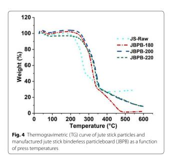
14.48%. This indicates that JBPB-220 has good thermal stability. These results revealed that JBPB-180 and JBPB-200 were thermally degraded faster compared to JBPB-220. The reason can be explained by the formation of hydrogen bonds due to hot pressing and with increasing of press temperature up to 220 °C auto-crosslinking polymer chains started [48] thus tough to be broken in JBPB-220 board which increases its stability.
