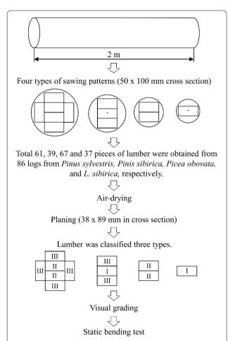
**Fig. 1** Illustration of the experimental procedures. I, lumber including pith at almost-center position in cross-section; II, lumber obtained near the pith (sometimes including pith on the surface area of the lumber); III, lumber obtained from outer part of the logs (without pith)
